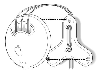
**Note:** The mounting bracket has enough space so that three cables (power, phone, and Ethernet) can be routed through it as shown in the illustration above, even though in most cases only two cables are used.
