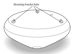
**4** Feed the cables through the mounting bracket and then connect them to the base station. The unit is designed to mount with the ports on the top (Apple logo right-side up), with the cables passing behind the unit through the mounting bracket as shown.
