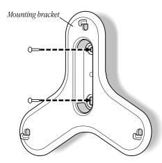
**3** Locate the three mounting bracket holes on the bottom of the base station.
