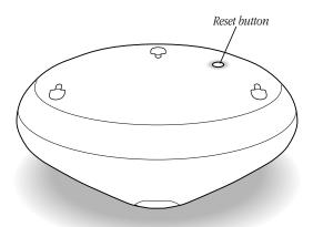
**2** Press and hold the reset button for one second.
