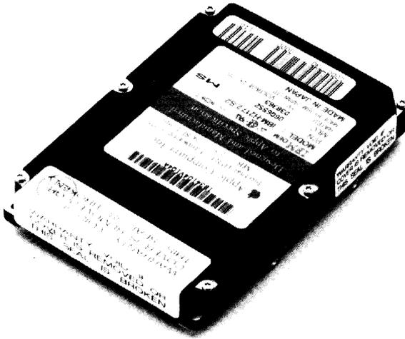
**NOTE:** The Apple Hard Disk 160 MB, 240 MB, and 320 MB, 2.5", SCSI drives are similar. You can identify the Apple Hard Disk 240 MB, 2.5", SCSI drive by the number *240 MB* on the drive label.
