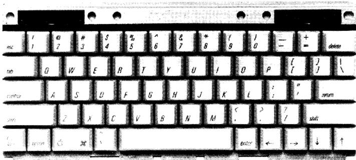
**NOTE:** The Macintosh Portable keyboard comes in two versions: the original keyboard (661-0476) has a steel mounting plate with a silver finish. The new keyboard (661-1612) has an aluminum mounting plate with a black finish. Also, the keyswtches are different and have a different feel. When replacing a keyboard, order the replacement module with the same mounting plate as the defective keyboard.
