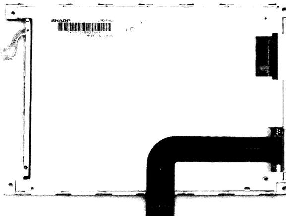
**NOTE:** Transfer the protective plastic from the new module to the module being returned.
