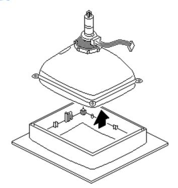
2 Caution: The neck of the CRT is easily damaged. Do not grab the neck of the CRT to remove it from the bezel. If necessary, have a helper hold down the bezel while you hold the CRT by its edges and remove it.
