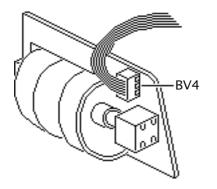
**Caution:** To avoid damaging the contrast/ brightness board, be sure to contact only connector BV4 cable wires with the soldering iron. Desolder one wire at a time, and remove as much solder as possible after desoldering each wire.
