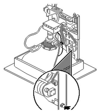
**A**Warning: Never use a grounding wriststrap until after discharging the CRT.
