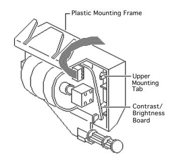
2 Push out on the upper mounting tabs, pull up on the cable, and remove the contrast/brightness board from the plastic mounting frame.
