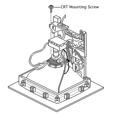
Using a Phillips screwdriver, remove the CRT mounting screw shown. Loosen but do not remove the other three CRT mounting screws.
