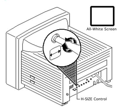
**Note:** Perform geometry adjustments whenever you replace the main board.
