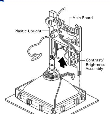
Grasp the contrast/ brightness assembly with one hand and the plastic upright on the left. Pull straight up and remove the main board.
