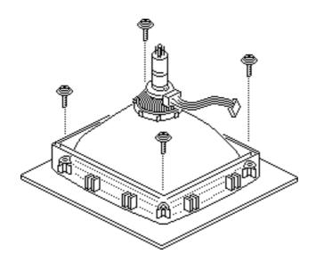
1 Remove the four screws that hold the CRT to the front bezel.
