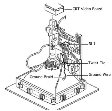
**Caution:** The neck of the CRT is easily damaged. Use caution when removing the CRT video board from the CRT neck. The cables between the board and the neck are very short.
