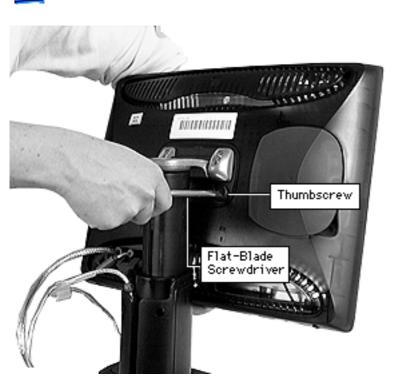
7 Using a flat-blade screwdriver, loosen but do not remove the two thumbscrews and thin plastic washers at the rear of the display.
