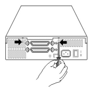
Using a jeweler's screwdriver, press gently on the two holding tabs as you push the case top up slightly.
