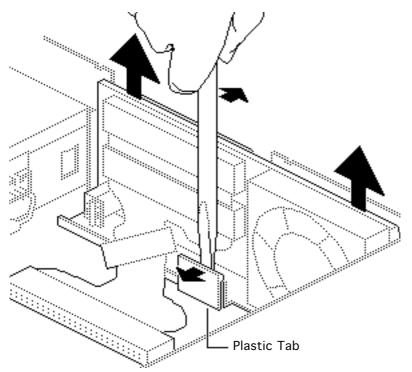
Using a flat-blade screwdriver, push back the plastic tab and lift out the metal fan frame (with fan, SCSI device-to-case cable, fan cable, and SCSI select switch attached).
