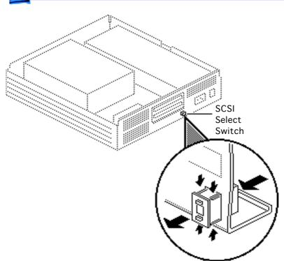
Depress the four plastic arms on the back of the switch and push the switch through the fan frame.
