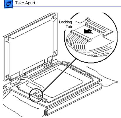
5 Using a small flat-blade screwdriver, pry up and disconnect the display cable.
