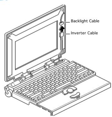
**Replacement Note:** To avoid pinching the inverter cable, make sure it routes as illustrated.
