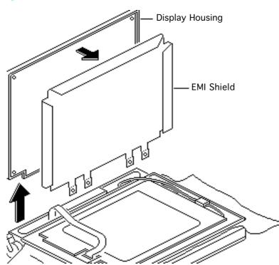
**Replacement Note:** To avoid pinching the inverter cable, make sure it routes as illustrated.
