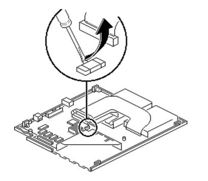
1 Using a small flat-blade screwdriver, pry up and remove the fuse.
