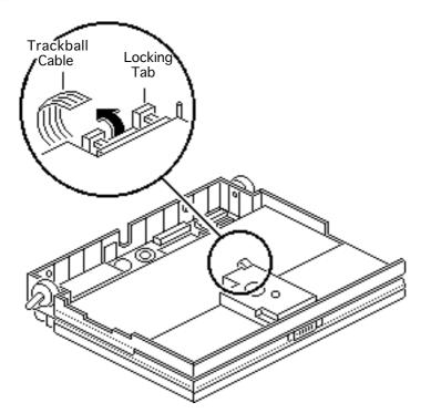
**Caution:** The trackball cable is fragile and should be handled with care.
