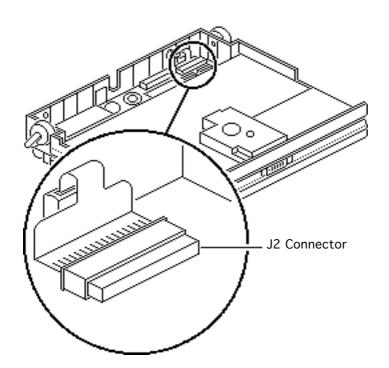
2 **Note:** The display cable will not come entirely out of the connector until you remove the interconnect board from the top case.
