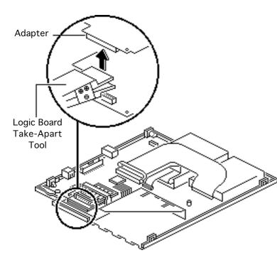
**Note:** To disconnect the adapter from the logic board, be sure to use the Apple logic board take-apart tool.
