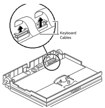
**Caution:** The keyboard ribbon cables are fragile and should be handled with care.
