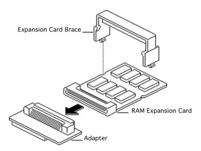
holding onto the white projections on the top of both cards and squeezing them together.
