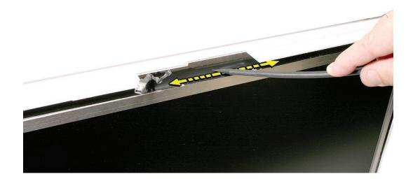
3. Wrap the cables with kapton tape then tuck the cables neatly into the channel on the rear housing.
