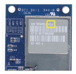
To locate the EEE code on the logic board, locate the memory slot inside the computer. Locate the last four digits in the serial number. Drop the last digit, in this case, the letter "A." The EEE code is the next three digits. In this case the EEE code is "WZH."
