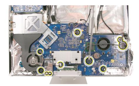
2. Using a T10 torx screwdriver, remove the screws from the logic board. The locations of the three self-tapping screws are marked by and "S" in the photo. The remaining three screws, are machine screws; they are marked with an "M". **Note**: Transfer the small metal grounding (located two screws below the battery) clip to the replacement logic board.
