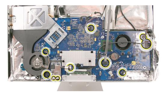
4. Secure the logic board by installing the machine screws first and then the self-tapping screws, marked with an "S".
