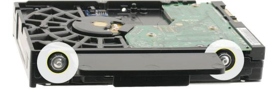
7. Using a T8 torx screwdriver, remove two mounting pins from the other side of the drive.
