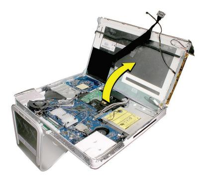
Note: If replacing a bad LCD display, you will need to remove the lower EMI shield (if still attached), the display panel mounting brackets, and the LVDS cable as follows.
