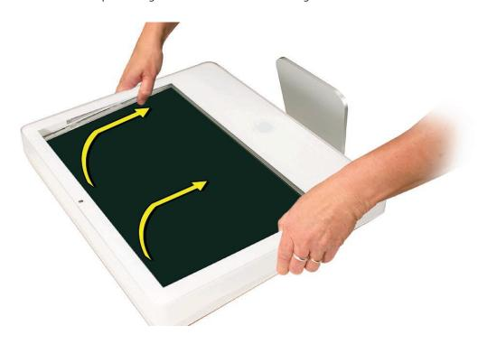
10. Lift the bottom of the front bezel straight up to remove it, and swing the bezel over onto its top edge. Disconnect the two cables attached to the top of the bezel.
