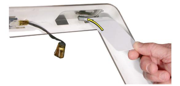
5. Start on the left side (looking from the back of the unit). Insert the card to disengage the latch. Squeeze the top of the bezel, that will help take pressure off of the latch and enable it to open easier. As the bezel releases, pull the bezel away from the rear housing.
