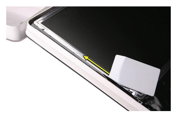
2. Using the access tool or black stick, peel back the black EMI tape stuck along the entire length of the top panel.
