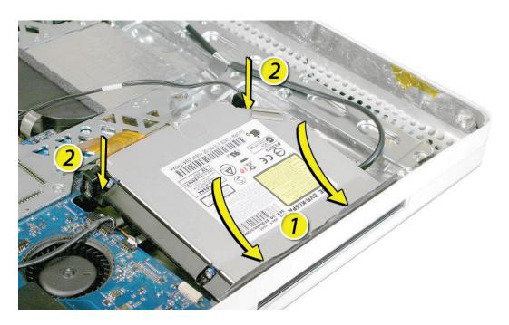
3. Connect the optical sensor cable to the logic board. Route the sensor cable under the optical flex cable. Connect the flex cable to the logic board and replace the T6 screws.
