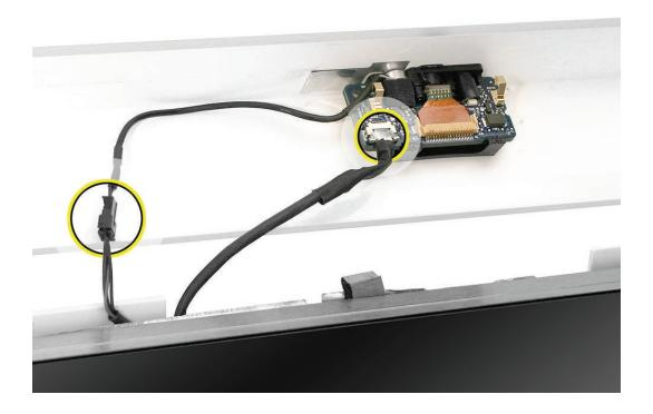
5. Tuck the camera board cables neatly into the channel on the rear housing.
