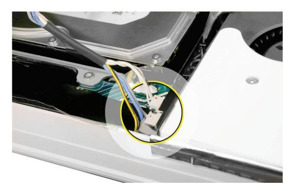
Raise the panel up the rest of the way. Disconnect the two inverter-to-display cables at the top of the inverter. Replacement Note: The cable connectors are marked with dots to indicate "right-side up."
