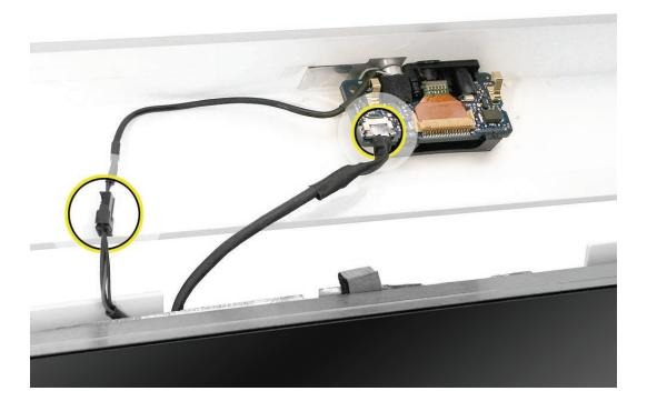
3. Tuck the cables neatly into the channel on the rear housing.
