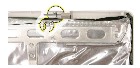
3. Remove any other tape that secures the antenna cables to the rear housing. Pull the antenna cable(s) through the access hole at the top of the EMI shield, near the antenna board.
