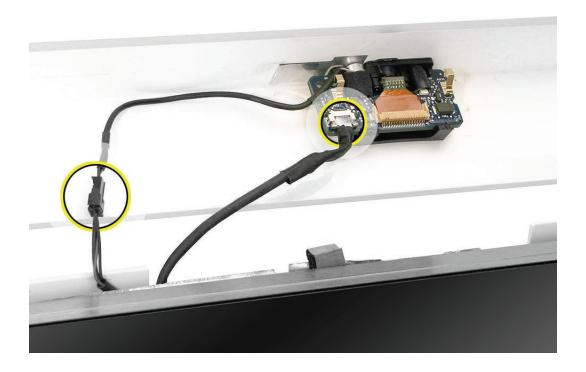
3. Remove any kapton tape covering the camera board. With your fingernail or a black stick, gently lift/flip up the flex cable locking hinge to release the flexible camera cable.
