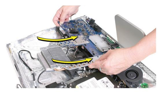
4. At the top of the heatsink, replace the two T6 screws attaching the logic board support bracket to the chassis. Note: The L-shaped support brackets must be transferred to the replacement logic board.
