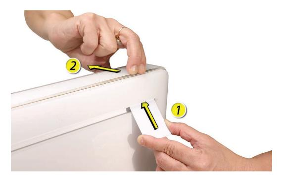
If the bezel won't release, pull the bottom of the bezel out a bit and insert the access card again.
