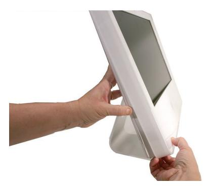
9. Once the access card has been removed, it is safe to open the bezel. Position the unit on an ESD mat, with the bottom facing toward you. Lift up the top of the bezel and pull it up and slightly toward you. Caution: Make sure the memory eject levers are not protruding from the access door when you lift the bezel up.
