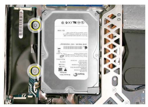
2. Disconnect the hard drive sensor cable from the connector on the logic board. Note the location of the sensor on the side of the hard drive and the routing of the sensor cable under the heat pipes.
