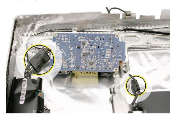
2. Replace the four power supply screws. Install the machine screw (bottom right corner) first when installing the power supply.
