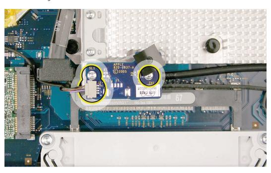
If necessary, use a Torx T6 screwdriver to remove the IR board mounting bracket.
