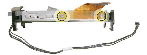
7. If replacing the optical drive, disconnect the sensor cable from the optical sensor located on the underside of the optical drive. Transfer the sensor cable to the replacement drive.
