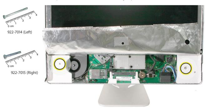
2. Remove the tow T6 screws on the IR mounting bracket so the speaker cable insulation is not sliced on the metal bracket.
