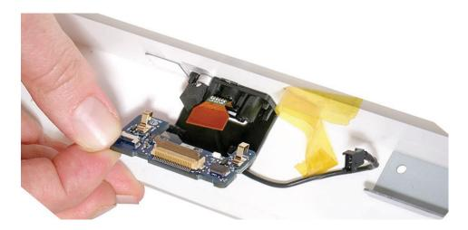
2. Snap the board into the mounting bracket and lock the flex cable into the connector with the locking hinge.
