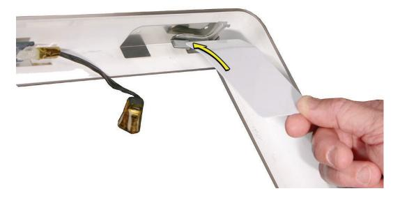
5. Start on the left side (looking from the back of the unit). As you insert the card to disengage the latch, squeeze the top of the bezel, that will help take pressure off of the latch and enable it to open easier. As the bezel releases, pull the bezel away from the rear housing. Note: If the bezel won't open, try cutting the card lengthwise into 3/4 inch or 1.5 cm strips. Insert the card on a 45° angle, aimed toward the outer corner, and try again.
