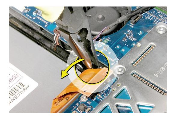
5. This photo shows the optical drive out of the computer so you can visualize how the clips move. Pressing down (#1) releases the clips (#2) outward from the metal chassis. Caution: Never press down on or grasp the body of the optical drive when removing or installing it. Pressing or squeezing the body of the optical drive could damage the mechanism.
