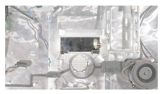
2. Peel back the EMI tape on top of the mechanism. Using a torx T10 screwdriver, remove the four clutch mounting screws.
