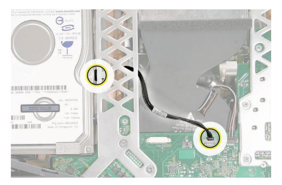
6. Connect the optical drive sensor cable, optical flex cable, optical clip, and replace the optical clip screws.
