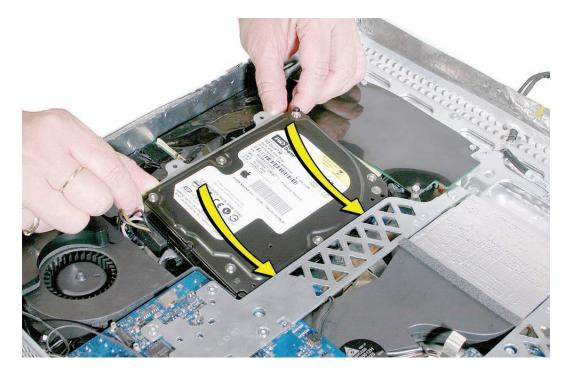
5. Secure the two T10 screws on the hard drive mounting bracket to the inverter board.
