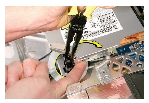
Warning: iMac main logic boards returned with physical damage such as scratches, fractures, or broken or missing components caused by improper servicing may be classified as customer abuse. When using a tool to release the latches, be careful not to apply pressure to the logic board or it may be damaged.
