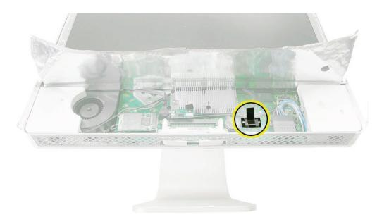
4. Using a Torx T10 screwdriver, remove the four panel mounting screws.
