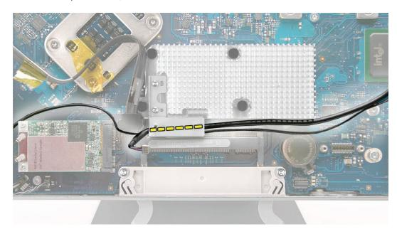
2. Install the IR board on the mounting bracket. Replace the T6 screws and connect the IR cable to the IR board.
