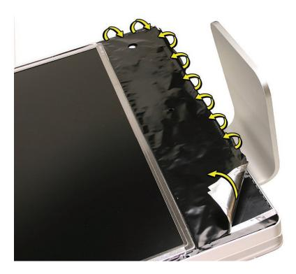
2. Gently lift the EMI shield to rest of the way to expose the other modules.
