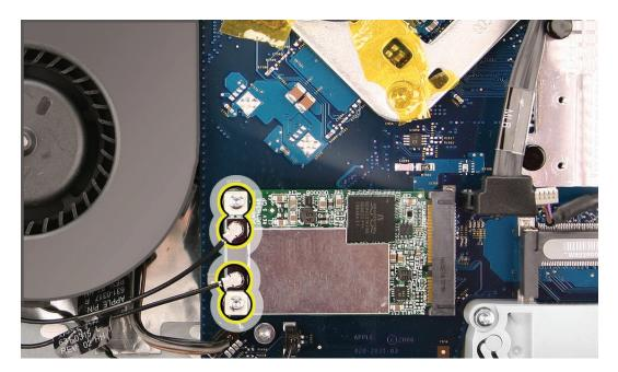
2. The board pops up when the screws are removed. Pull the AirPort Extreme card out of the slot in the direction of the arrow.
