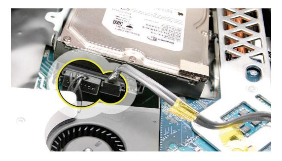
5. If you are replacing the hard drive, transfer the temperature sensor, mounting pins, and the metal mounting bracket to the replacement drive.
