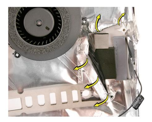
2. Using a black stick, pry the antenna board off the rear housing.
