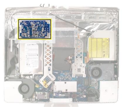
WARNING: The AC/DC power supply PCB remains powered up whenever the system is plugged in, whether or not the system has been turned on. Use extreme caution when troubleshooting the system with the front bezel removed.
