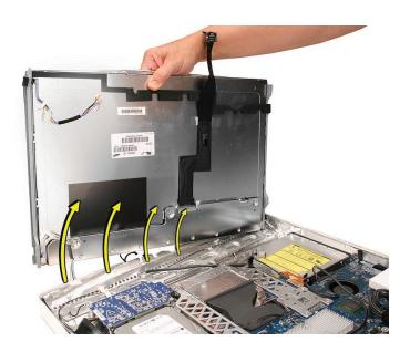
9. **Note**: If replacing the display panel, remove the lower EMI shield, the display panel mounting brackets (on each side), and the LVDS cable from the back of the display panel before returning the module to Apple.
