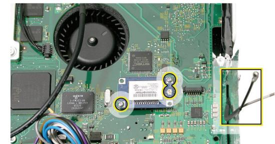
2. Lift the card off the logic board.
