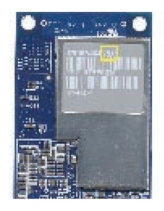
To locate the EEE code on the logic board, locate the memory slot inside the computer. Locate the last four digits in the serial number. Drop the last digit, in this case, the letter "A." The EEE code is the next three digits. In this case the EEE code is "WZH."
