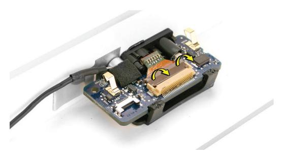
4. With your fingers or black stick, flex the two black tabs forward to release the camera board from the camera bracket.
