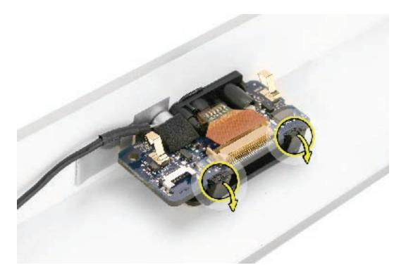
5. Remove the camera board from the front bezel. **Note**: The flex cable, camera lens, and black mounting bracket are part of the front bezel.
