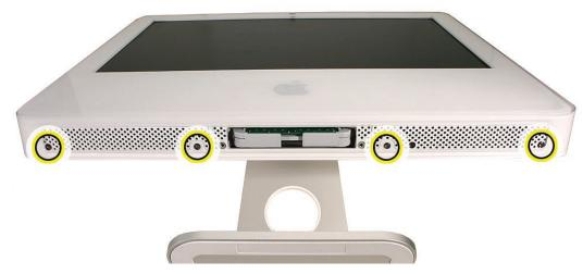
3. Locate the access card. Bending the upper quarter of the access tool card will help engage the latch. Note: Refer to Access Tool Modification in the General Information chapter if the bezel is difficult to open.
