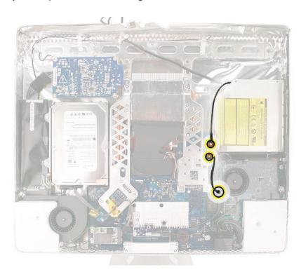
2. **Note**: Make sure to use a needlenose pliers with teeth to remove the optical drive. The pliers must have a textured surface to properly grasp the optical drive release tabs.
