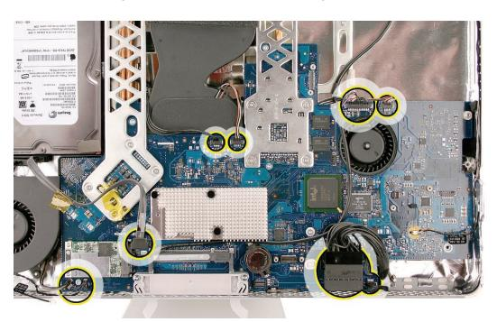
2. Remove seven T10 screws. Screws are labeled below as self-tapping or machine screws.-
