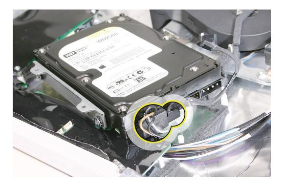
3. Route the hard drive sensor cable under the metal chassis. Connect the sensor cable to the logic board.
