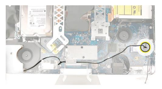
Lift the speakers up and out of the computer. See the next photo for disconnecting the speaker.
