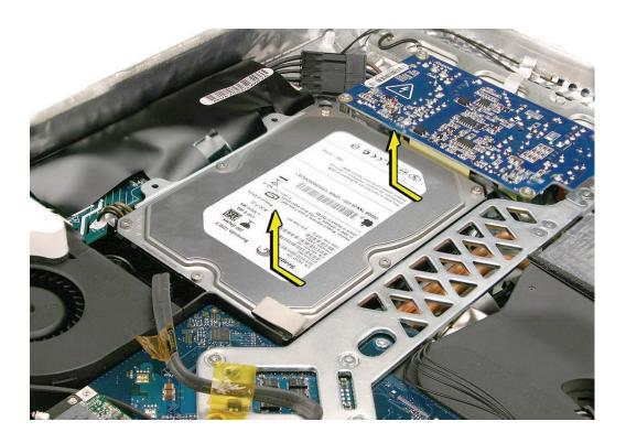
Disconnect the hard drive power and data cables from the end of the hard drive.
