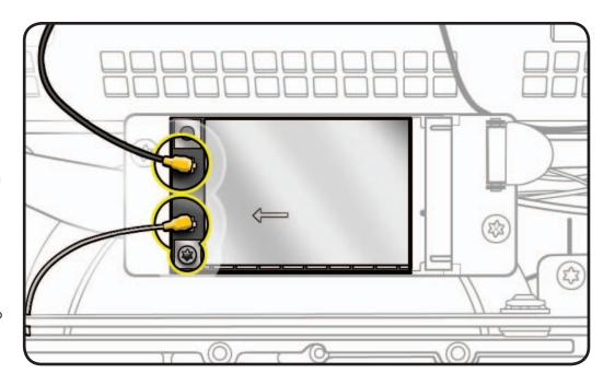
**3** Hold AirPort card by edges and pull it out of the slot.
