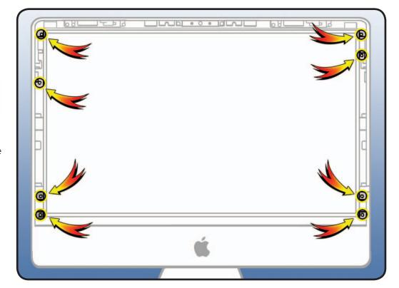
**2** With computer standing up and facing you, pull the LCD forward slightly from the top edge to access cables inside.
