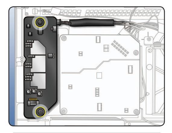
2 Lift up board, flip over, and disconnect power connector.
