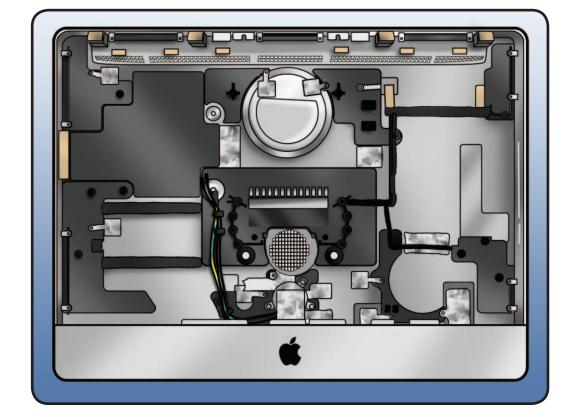
With all other modules removed, rear housing is the remaining assembly.
