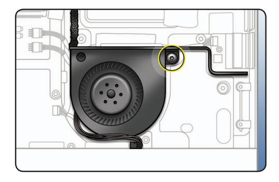
2 Lift fan up and disconnect cable from logic board.
