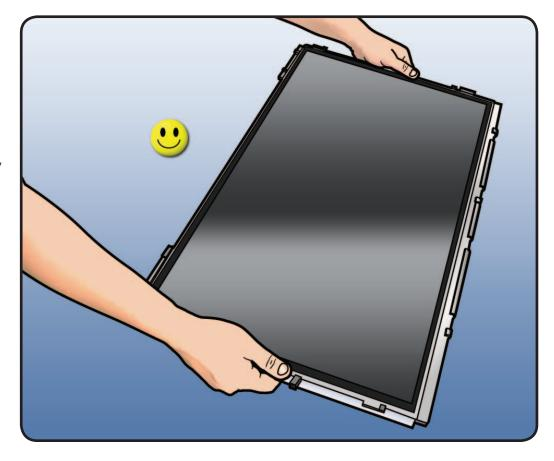
2 Never touch LCD surface or hold LCD panel with one hand. It could damage the LCD panel.
