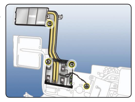
4 (1) Lift up video card and heatsink and (2) slide card out of slot on logic board.
