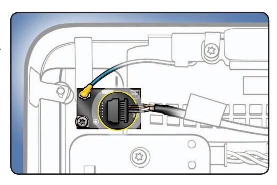
2 Disconnect cable (#5) from top center of logic board.
