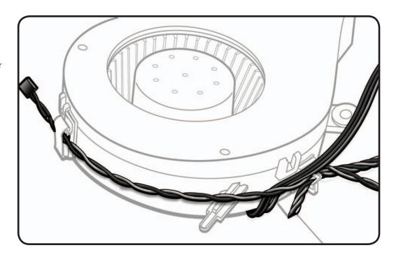
**3** Note routing of cable and any tape securing it to rear housing.
