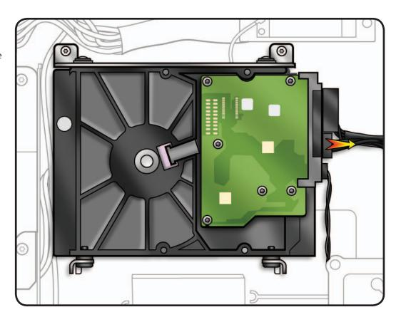
2 Disconnect hard drive data cable (#19) from back side of logic board.
