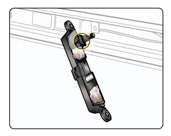
2 Disconnect cable (#6) from top center of logic board.
