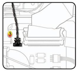
LEFT: Close-up of #2 backlight power cable at bottom of LED backlight board. Pinch and pull cable down from connector.
