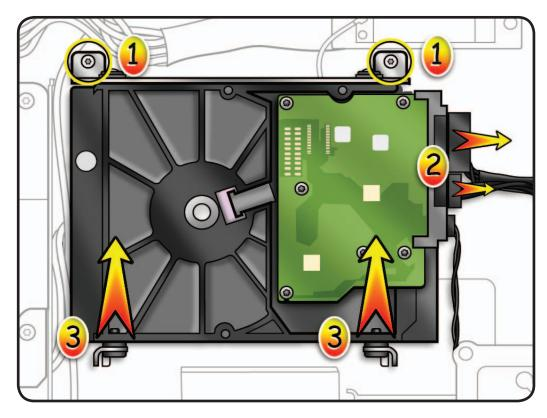
Disconnect HD sensor cable from top of logic board.
