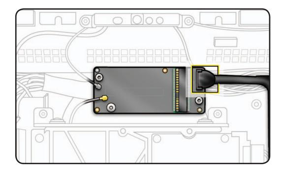
2 Disconnect cable (10) from top center of logic board.
