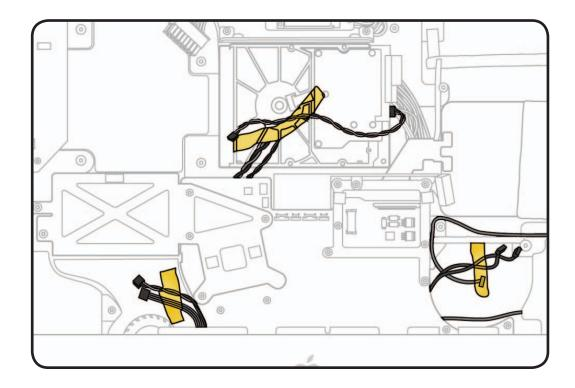
**6** Peel up foil holding copper square to rear housing.
