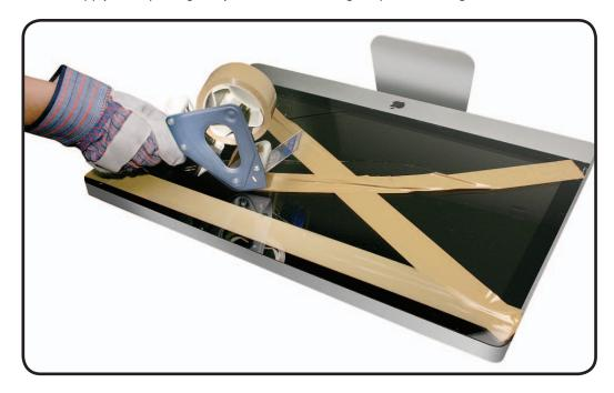
5. Continue applying tape horizontally, thoroughly covering the broken glass. Most of the glass will still be attached to the steel ring that runs around the perimeter of the glass panel.
