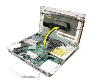
Note: If replacing a bad LCD display, you will also need to remove the lower EMI shield (if still attached), the display panel mounting brackets, and the LVDS cable as follows.
