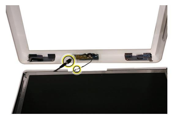
12. If replacing a damaged front bezel, remove the camera board.
