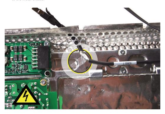
3. Route the camera cable as shown, and tape the camera cable and DC power cable to the rear housing as shown below.
