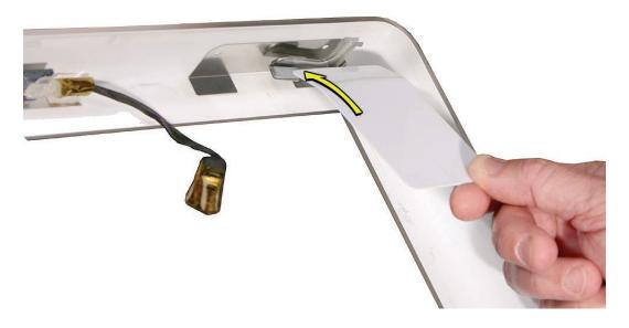
5. Start on the left side (looking from the back of the unit). As you insert the card to disengage the latch, squeeze the top of the bezel, that will help take pressure off of the latch and enable it to open easier. As the bezel releases, pull the bezel away from the rear housing. Note: If the bezel won't open, try cutting the card lengthwise into 3/4 inch or 1.5 cm strips. Insert the card again, on a 45° angle, aimed toward the outer corner, and try again.
