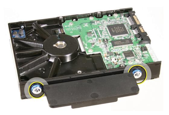
7. Using a T8 torx screwdriver, remove two mounting pins from the other side of the drive.
