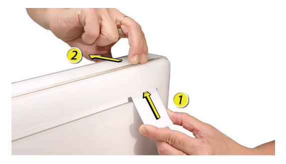
7. If the bezel won't release, pull the bottom of the bezel out a bit and insert the access card again.
