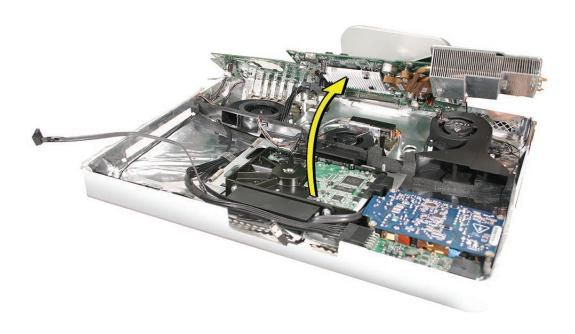
5. Disconnect the power supply cable and carefully lift the logic board out of the chassis.
