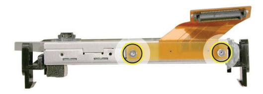
7. If replacing a bad optical drive, remove the temperature sensor from the top of the drive. Discard the sensor—the replacement drive comes with a new sensor already installed.
