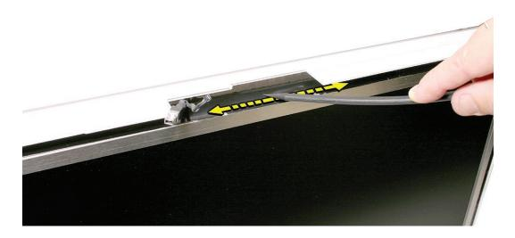
3. Tuck the cables neatly into the channel on the rear housing.
