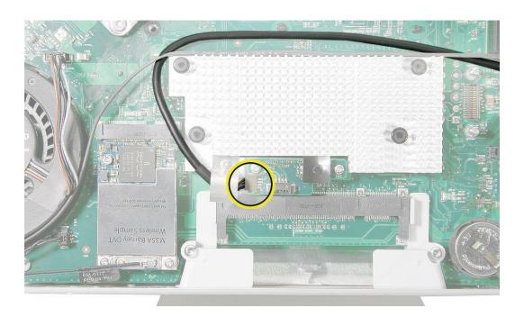
2. Using a Torx T6 screwdriver, remove the two IR board screws. Remove the IR board from its mounting bracket.
