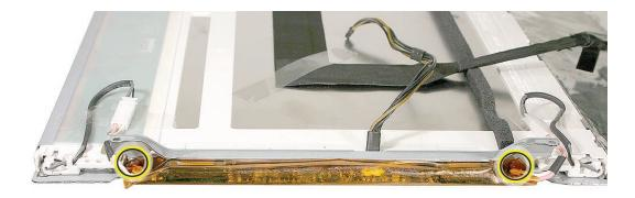
8. Peel back the tape where shown below, and disconnect the two inverter-to-display cable connectors.
