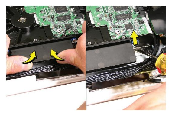
4. Disconnect the hard drive power and data cables. Lift the hard drive out of the chassis.
