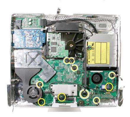
2. Using a T10 torx screwdriver, remove the screws from the logic board. Note the locations of the self-tapping and machine screws as you remove the screws.
