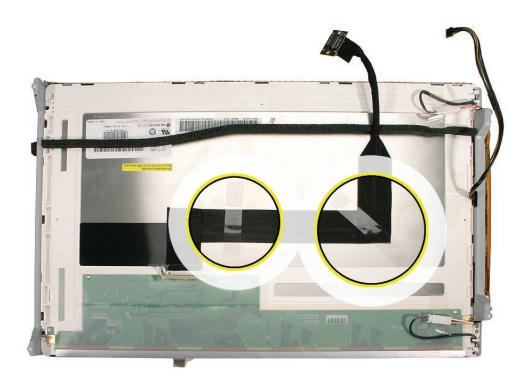
2. Pinch together the connector locking levers, and disconnect the LVDS cable connector.
