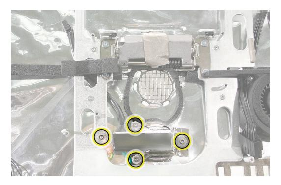
3. Peel the EMI tape off the AC filter.
