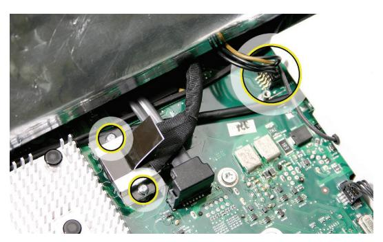
3. Peel the EMI tape away from each side of the panel. Using a Torx T10 screwdriver, remove the four panel mounting screws.
