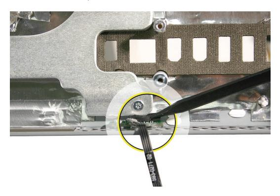
2. With a black stick, pry the ambient light sensor board from the frame.
