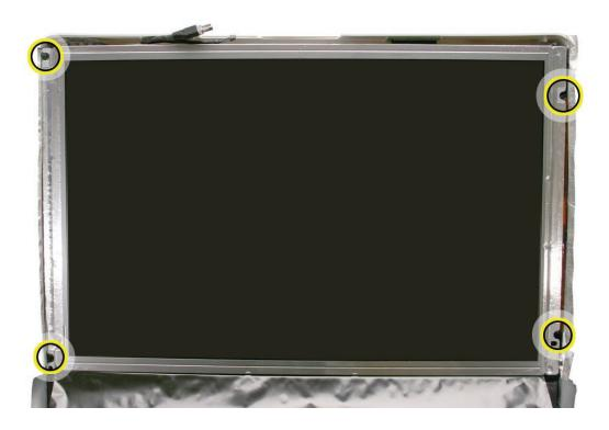
4. Pivot the panel up, as shown, then carefully peel the top edge of the panel away from the EMI shield.
