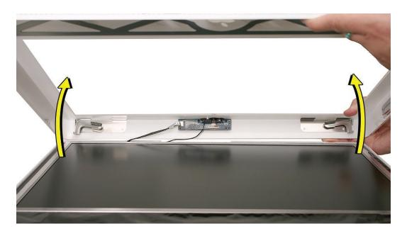
2. Disconnect the camera and microphone cables.
