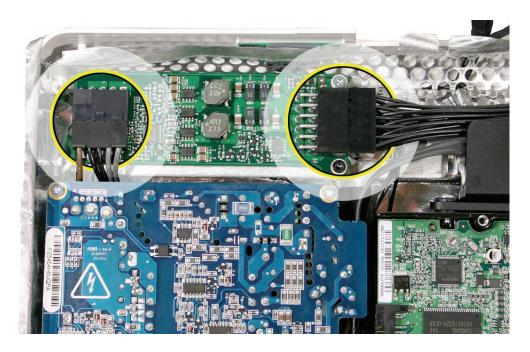
2. Using a T10 torx screwdriver, remove the self-tapping screw from the top corner of the DC-DC board and the black self-tapping screw below it. Lift the board straight up to remove it.
