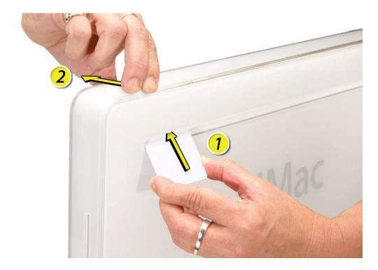
6. Repeat step 5 to release the locking latch in the right corner. Again, pull the bezel away as the card releases the latch.
