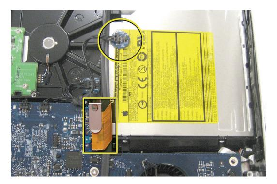
2. Note: Make sure to use a needlenose pliers with teeth to remove the optical drive. The pliers must have a textured surface to properly grasp the optical drive release tabs.
