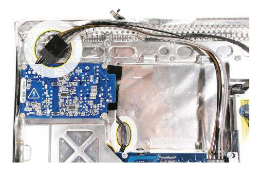
2. Using a T10 screwdriver, Remove the T10 AC power inlet ground-to-chassis screw.
