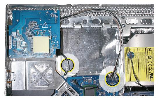
2. Rotate the computer so that the stand is away from you. Locate the power supply connector underneath the logic board. Use a black stick to release the connector.
