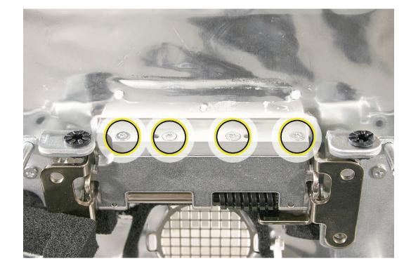
3. Using a T10 torx screwdriver, remove the four clutch mounting screws.
