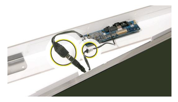
3. Using a T6 screwdriver, peel back the mylar and kapton tape as necessary and remove the two camera board mounting screws. Pull the camera board straight out of the lens aperture in the bezel to remove it.
