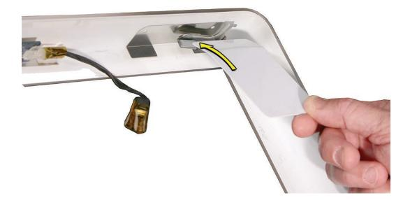
5. Start on the left side (looking from the back of the unit). Insert the card to disengage the latch. Squeeze the top of the bezel, that will help take pressure off of the latch and enable it to open easier. As the bezel releases, pull the bezel away from the rear housing.
