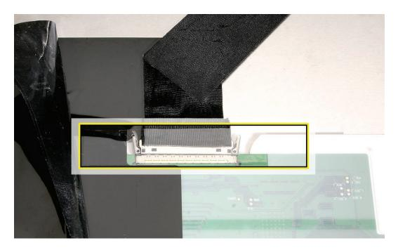
3. If you are replacing the display, a piece of black mylar is enclosed in the box with the display module. The dotted lines below show the correct placement of the mylar. **Note**: The LVDS locking lever (on one side) should be covered by the mylar when positioned correctly.
