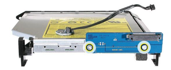
7. If replacing a bad optical drive, also remove the temperature sensor from the top of the drive. Discard the sensor—the replacement drive comes with a new sensor already installed.
