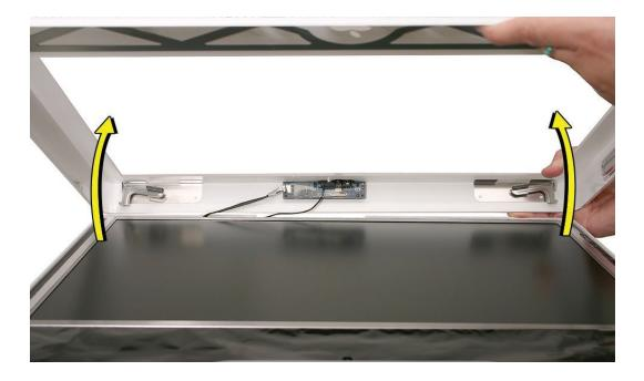
2. Disconnect the camera and microphone cables.
