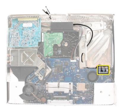
2. Disconnect the camera cables and pull the cable through the access hole at the top of the EMI shield. Remove the camera cable from the rear housing.
