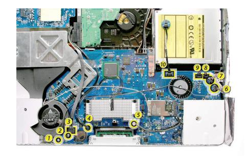
2. Using a T10 torx screwdriver, remove the screws from the logic board. Note the locations of the three self-tapping screws (marked by and "S" in the photo). The rest of the screws are machine screws.
