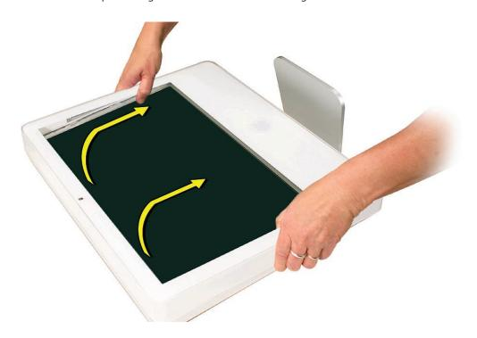
10. Lift the bottom of the front bezel straight up to remove it, and swing the bezel over onto its top edge so you can disconnect two cables attached to the top of the bezel.
