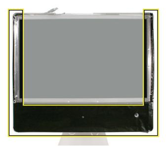
Pay particular attention to the EMI shielding inside the rear housing, shown below. The EMI shield is easily damaged when replacing modules
