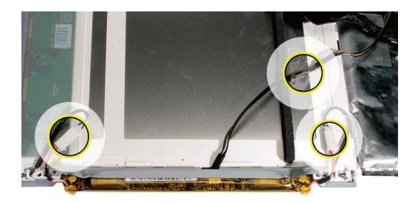
2. Using a flat-blade screwdriver as shown, pry up the inverter to remove it from inside the display panel mounting bracket.
