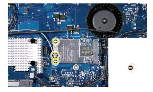
2. The card will spring up when the screws are removed. Grab the card from the connector end, pull the card from its socket on the logic board.
