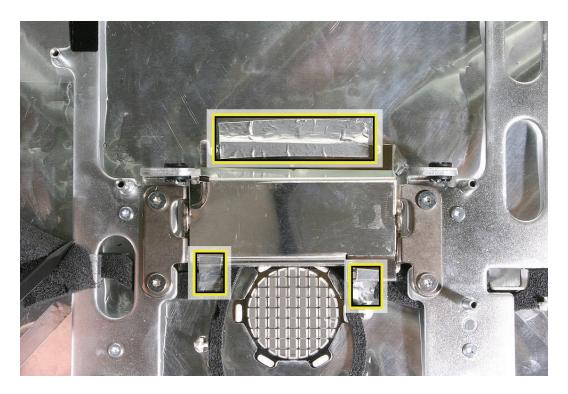
2. Remove the metal clutch cover.
