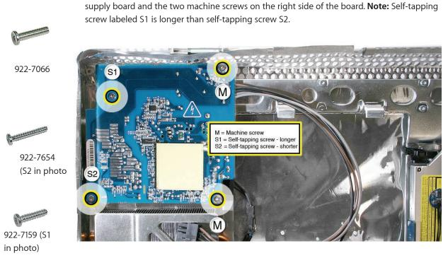
3. Using a T8 screwdriver, remove the two self-tapping screws on the left side of the power
