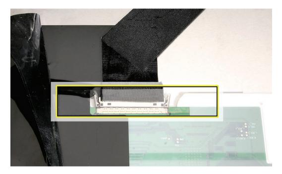
4. Replace the display panel. **Note**: If you are replacing the display, a piece of black mylar is enclosed in the box with the display module. The dotted lines below show the correct placement of the mylar. The LVDS locking lever (on one side) will be covered by the mylar when positioned correctly.
