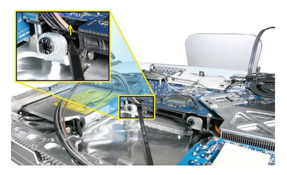
4. Pull the board toward you and slightly lift the board up. **Note**: The I/O ports fit tightly into the port hole openings on the rear cover. You may have to fidget with the board a bit to free the ports from the rear cover. Remove the logic board out of the rear housing.
