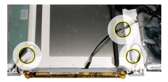
8. To access the LVDS cable connector, peel back the black mylar tape that partially covers the LVDS connector.
