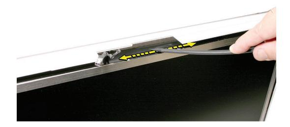
3. Tuck the cables neatly into the channel on the rear housing.
