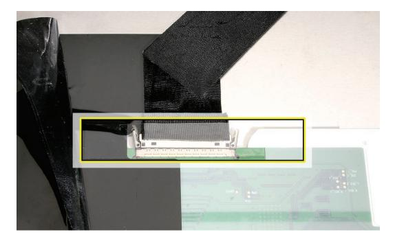
3. Pinch together the connector locking levers, and disconnect the LVDS cable connector.
