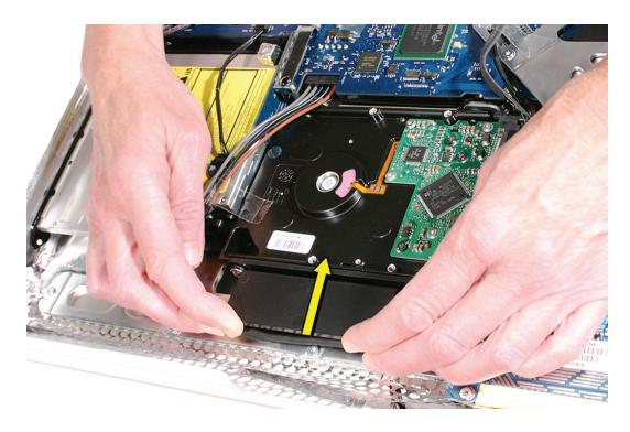
3. Disconnect the hard drive power and data cables. Set the hard drive aside.
