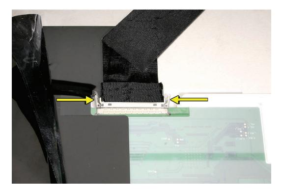
10. Pinch together the connector locking levers, and disconnect the LVDS cable connector.
