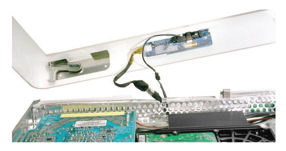
2. Route the camera cable around the hard drive and under the chassis (as shown). Connect the two cables to the connectors on the logic board.
