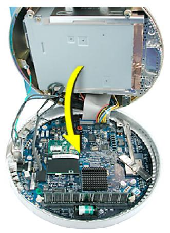
Important: Diagnostic service cables allow the unit to run while the bottom housing is open (as shown above). However, the computer cannot run for more than five minutes with the bottom housing open. If it is open longer, the CPU may overheat and become damaged.
