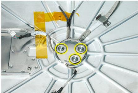
3. Loosen the four screws (shown below) that hold the panel shield to the neck assembly, and tilt the screen the opposite direction of the tilt.
