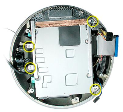
4. With the drive door still positioned at the top, look for the white plastic clip attached to the side of the drive carrier. Open the clip and remove the Airport antenna and the video cable from the cable clip.
