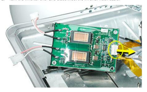
3. Remove the inverter from the display support shield.
