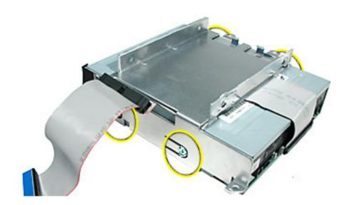
10. Slide the optical drive out of the carrier. Be careful of the black plastic dust filter on the carrier. It is very fragile and can rip easily if not handled properly. Note: The silver insulator is part of the carrier assembly.
