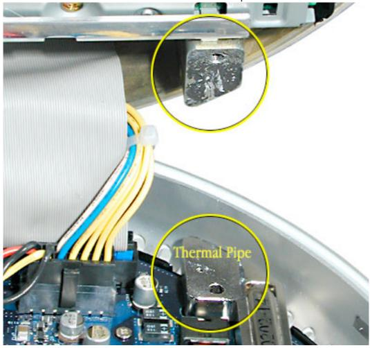
2 Squeeze a drop of thermal paste onto the middle of the thermal pipe surface as shown below. **Note:** In testing, the drop of thermal paste shown below completely covered the entire thermal pipe surface. Place <u>at least</u> this much paste on the thermal pipe.
