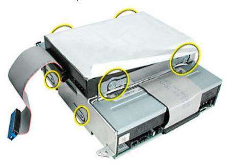
17. Replace the optical/drive carrier assembly, EMI shield, and screws.
