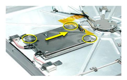
2. Turn the inverter over and disconnect the inverter neck cable.
