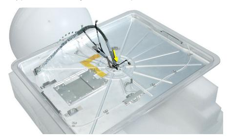
4. Line up the notches on the panel shield hole with the video cable. Gently pull the video cable through the panel shield (See next graphic for a close-up of the video cable going through the hole). Lift the shield off the back cover being careful not to scratch the white coating on the back cover.
