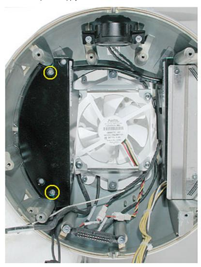
Open the optical drive door as shown to locate the two hidden screws near the drive door. Remove the four screws. Note: Support the metal plate and power supply as you remove the screws.
