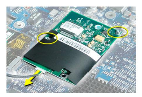
2. Lift the modem from the connector on the logic board.
