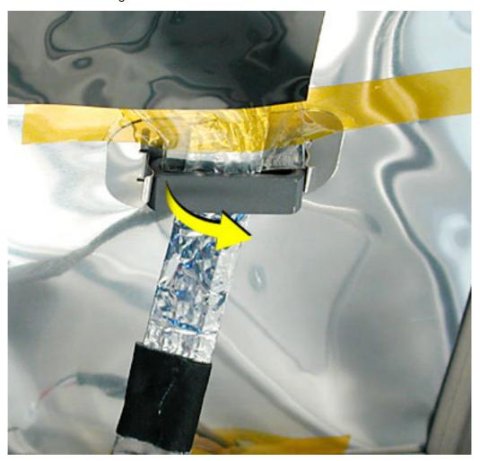
7. Lift the flat panel off the back cover. You are left with the LCD flat panel service part.
