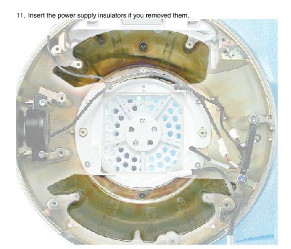
12. Replace the fan, the fans screws, and connect the fan cable.
