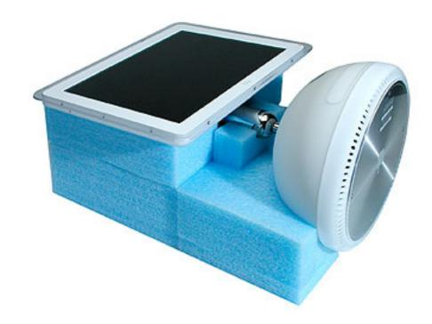
1. Support the computer by neck and the base (A). Gently position the computer in the service stand with the flat panel facing up (B).
