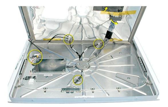
6. This shows a close up of the video cable, ferrite bead, and video cable clip. After removing the tape, carefully use a screwdriver to pry the ferrite bead from the video cable clip. Pry the ferrite bead from the side or from the back. Note: The ferrite bead is fragile and could break if a screwdriver is placed in the middle of the ferrite bead and is used as leverage to remove the bead.
