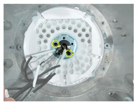
6. Route the neck cables in the base (as shown) and replace the three silver screws in the neck cap retainer.
