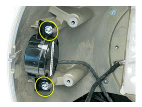
8. Attach the blind mate connector and screws. Remember, the tab on the blind mate connector faces inward.
