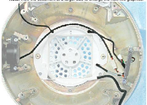
2. Loosen the three silver screws (circled below) to remove the neck cap. Lift the cap off the spokes. **Note:** The two black screws keep the neck attached to the base.
