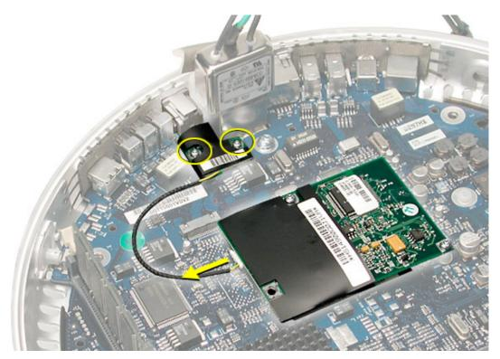
2. Remove the RJ-11 board from the I/O port.
