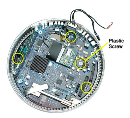
2. Grab the logic board by the battery retainer and the hard drive connector. Lift the board and pull back to release the board from the bottom housing and I/O ports. Note: The I/O port covers may come out with the logic board when it's removed.
