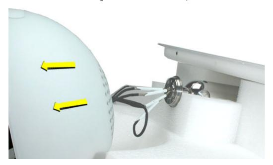
5. Replace the two black neck cap screws to connect the neck to the chassis.
