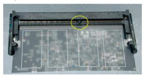
Important: Do not push the clips (circled below) when inserting memory. They are
