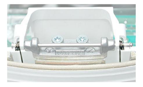
4. Remove the door hinge screws.
