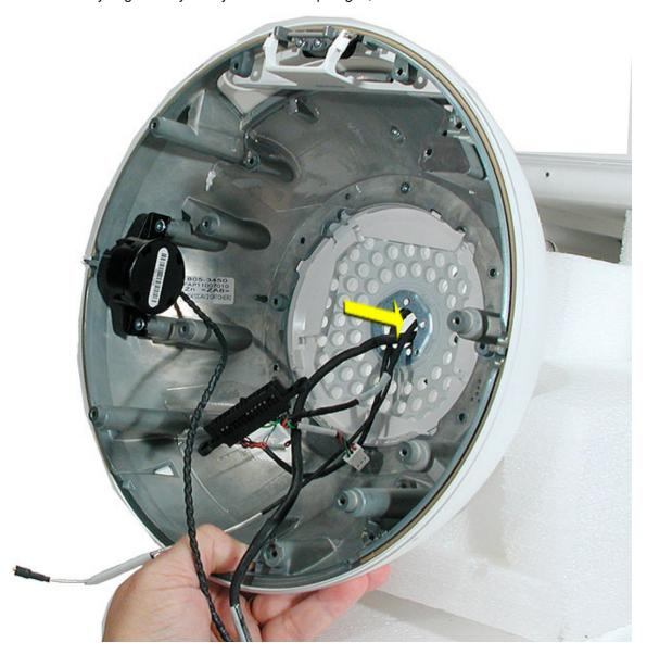
4. Pull the outer shell (with Faraday attached) away from the neck. Note: There is no need to remove the outer shell from the Faraday unless you are replacing a scratched or damaged outer shell. If you are removing the shell from the Faraday cage, go on to the next step.
