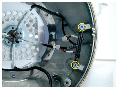
2. Lift the blind mate connector off the chassis. Note: The blind mate connector is part of the neck assembly.
