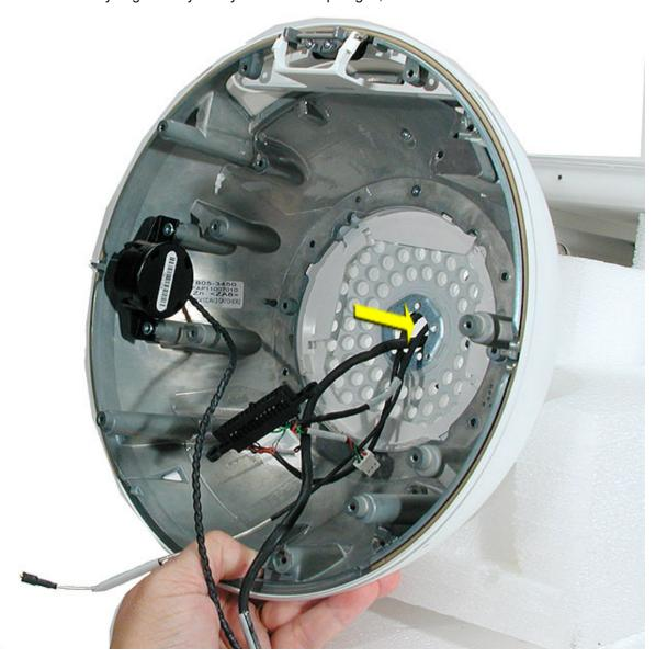
2. Pull the outer shell (with Faraday attached) away from the neck. **Note:** There is no need to remove the outer shell from the Faraday unless you are replacing the outer shell. **Important:** Be careful not to scratch the white paint on the inside of the housing shell and the metal neck plate (with holes).
