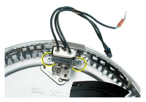
22. Replace the antenna extension and the black insulator into the bottom housing
