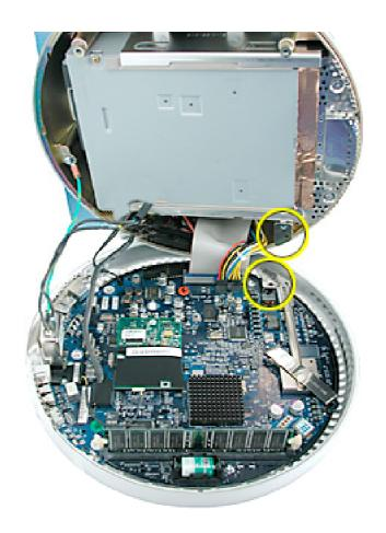
Thoroughly clean the original thermal film from the mating surfaces (circled below) of the bottom housing and thermal pipe. Use a plastic stylus to scrape the surfaces clean. Note: Do not use an abrasive material or liquid cleaner.
