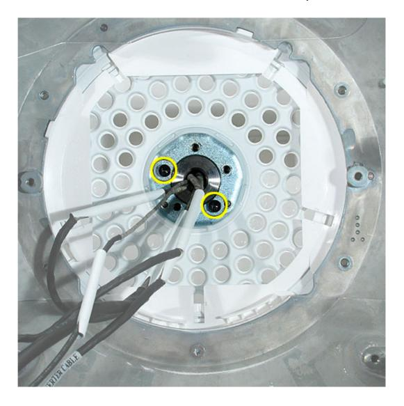
3. Carefully feed the neck cables through the hole in the Faraday cage. **Important:** The Faraday cage is very heavy and has sharp edges; handle with care.
