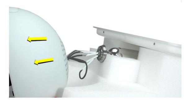
5. **Note:** Perform this step only if you are replacing the outer shell. Remove the three screws in the base of the Faraday cage to separate the shell from the Faraday cage.
