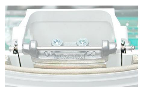
15. Rotate the base so the optical door is on the right. Replace the power supply and the six screws. Remember, the two smaller screw locations are hidden under the optical door flap.
