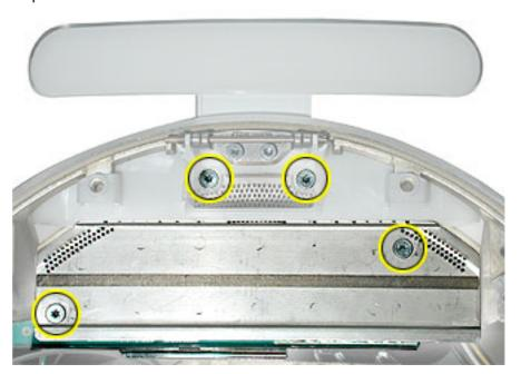
2. Slide the plastic door frame off the chassis.
