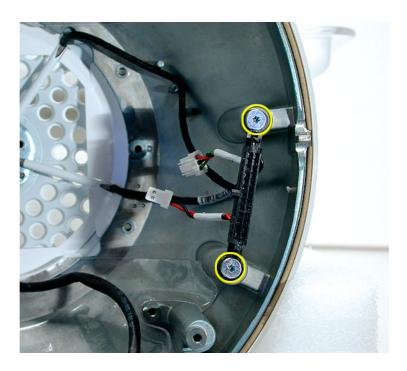
9. Attach the cable retainer and screws.
