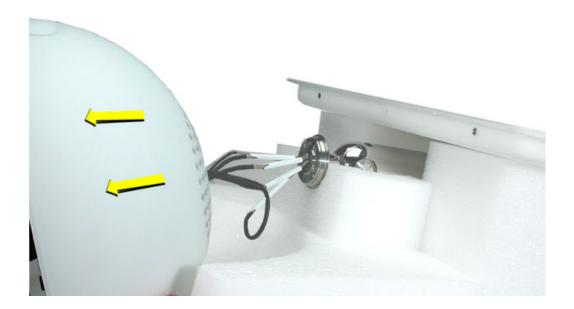
3. Remove the three screws in the base of the Faraday cage to separate the shell from the Faraday cage.
