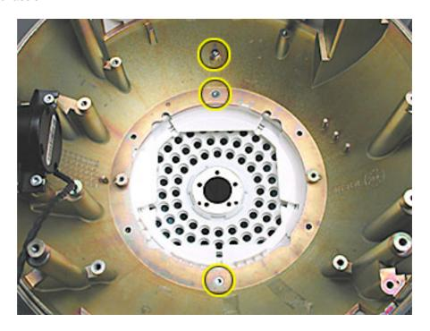
4. Thread the neck cables through the hole in the metal neck plate.
