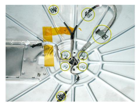
3. Gently pull the cables through the hole in the panel shield.
