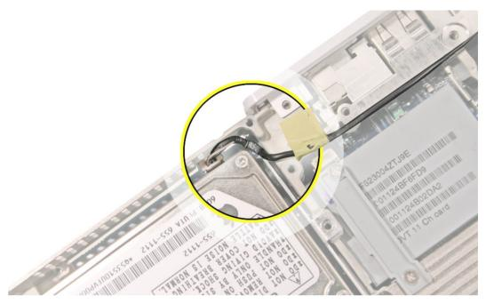
5. Press in on the upper bracket to clear it from the frame. While pressing on the bracket, use a black stick to begin to lift up the end of the hard drive.
