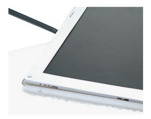
3. Lift off the display assembly from the display housing.
