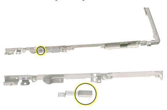
5. Install the replacement bezel brace with clutch assembly, and reassemble and test the computer.
