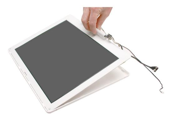
4. Install the replacement display rear housing, and reassemble and test the computer.
