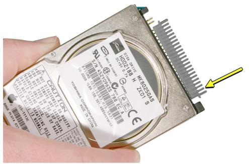
• Important: When setting the drive onto the logic board connector, tilt the drive slightly so that the connector slots align properly. Then level the drive, and make sure the brackets fit into the frame so that the grommets on the brackets match up with the holes in the frame. With the drive aligned properly, press on the connector to make sure it is fully engaged on the logic board.
