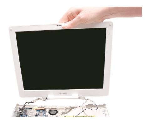
15. Install the display module, and reassemble and test the computer.
