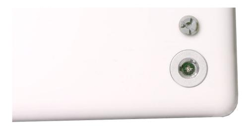
5. **Important:** To avoid damaging the case, be careful that the screwdriver tip does not slip out of the screw head during removal.
