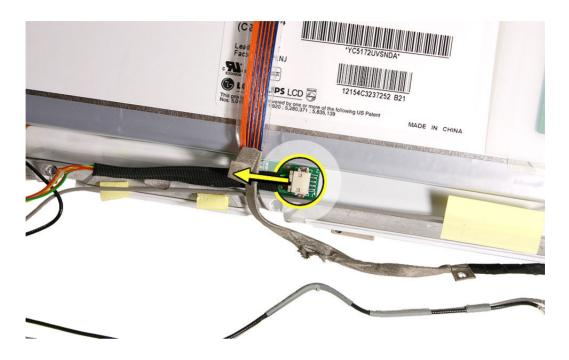
5. Install the replacement inverter cable and tape, and reassemble and test the computer.
