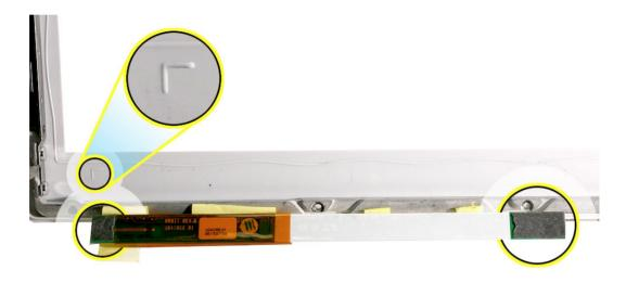
4. Install the replacement inverter board and cable, and reassemble and test the computer.
