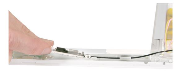
7. From the bottom of the bezel, lift up the inverter cable where the mesh tab anchors the gray antenna cable between the bezel brace and the inverter board.
