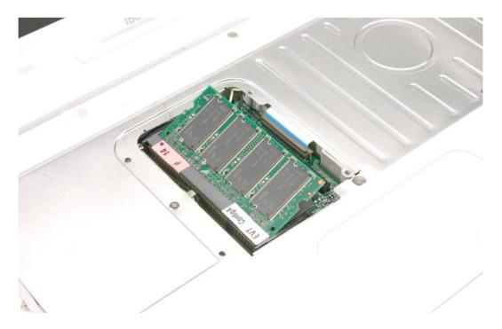
4. Align the notch in the replacement memory card with the small tab in the memory slot. Hold the card at a 30-degree angle, then push the card into the slot until it is firmly seated.
