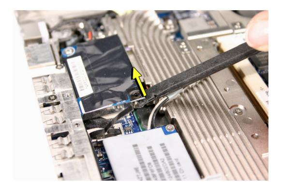
6. Disconnect the cable from the end of the modem board.
