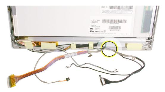
2. Peel up any tape that secures the microphone cable to the bottom of the bezel brace.
