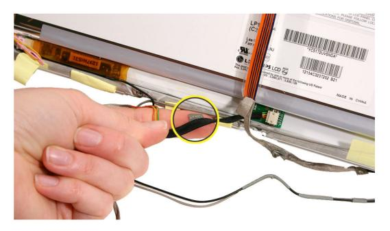
4. Use a black stick or flat-blade jeweler's screwdriver to disconnect the inverter cable from the inverter board.
