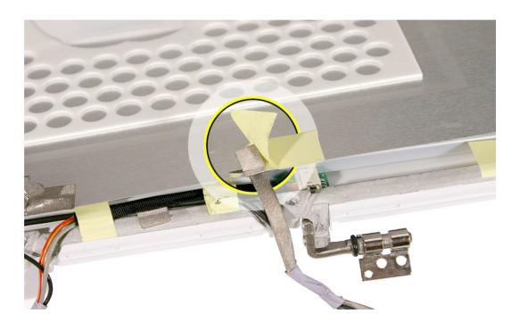
8. With the tape around the borders of the shield loosened or removed, lift up the shield, being careful not to bend it. Be careful if the foil tape catches on the LVDS cable.
