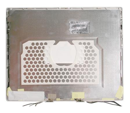
2. Near the right and left ends of the clutch cover, remove the two 12-mm long screws that secure the clutch cover to the hinge assembly.
