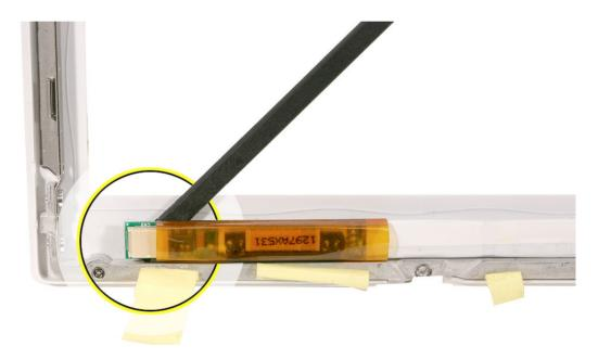
3. Pry up the board at the other end, and remove it from the bezel.
