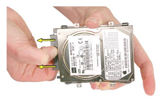
**Important:** If the hard drive pins become bent, use a black stick or jeweler's flatblade screwdriver to carefully straighten the pins.
