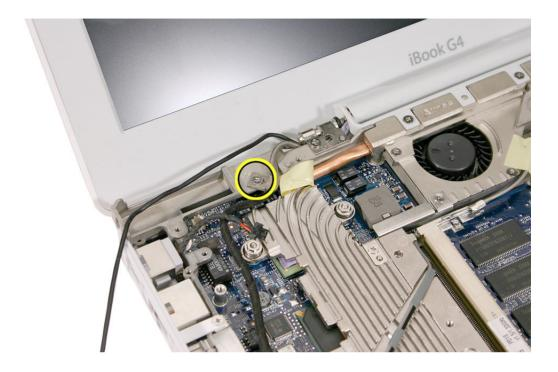
7. Holding the connector end of the AirPort Extreme/Bluetooth antenna cables, carefully lift them up from the corner space between the heatsink and the memory card slot.
