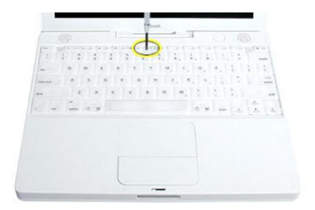
3. Release the keyboard by pulling down on the keyboard release tabs (located to the left of the F1 and F12 keys), then lift the top portion of the keyboard up slightly, and toward the display.
