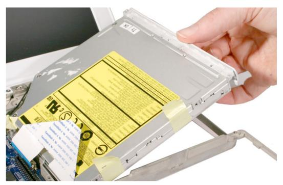
6. When removing the drive, the bottom of the drive case might stick to tape on the underside of the frame. If it does, use a black stick to release the drive.
