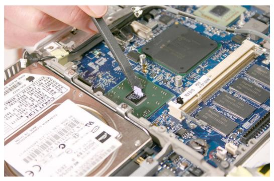
10. Install the replacement heatsink and new thermal pads, and reassemble and test the computer.
