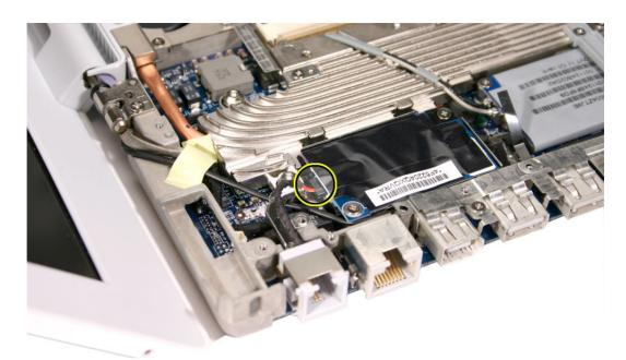
4. Use a black stick or needlenose pliers to disconnect the RJ11 modem cable from the modem board.
