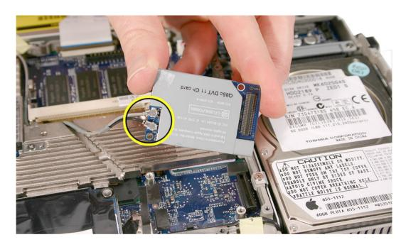
7. Disconnect the cables by pulling the connectors straight off the card.
