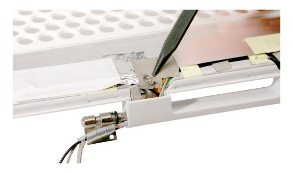
3. Tilt up the display assembly and pull straight down on the display clutch cover to remove the clutch cover from the display assembly.
