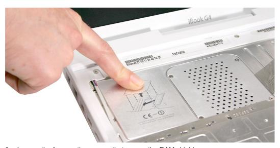
6. Loosen the four captive screws that secure the RAM shield.
