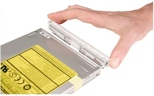
12. Install the replacement optical drive, and reassemble and test the computer.
