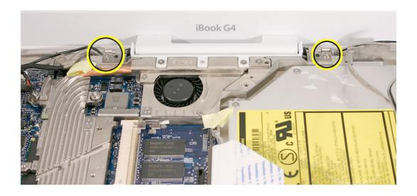
14. Warning: When lifting the display, be careful not to strain the cables.
