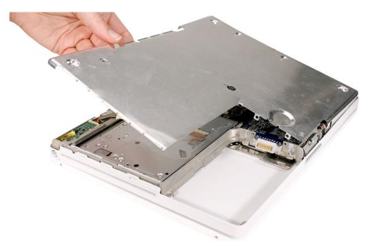
4. Note: The two springs in the battery compartment can become loose. When reassembling the computer, make sure that the two springs are in place before installing the bottom case. Each spring has grease on the coils, and each has a plastic cap on one end. Make sure the cap fits securely on the spring, and the curved side of the cap is positioned against the inner frame.
