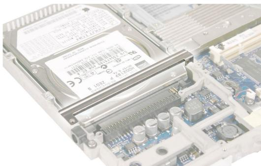
**Important:** Some optical drive flex cables carry the potential of an electrical short that would manifest as an optical drive error. Whenever you remove the top shield from this computer, be sure to check the optical drive cable and replace it, if necessary. For complete instructions, refer to the procedure "Checking the Optical Drive Cable" in the Additional Procedures chapter.
