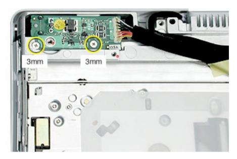
5. Tilt up the DC-in board, and pivot it out of the frame.
