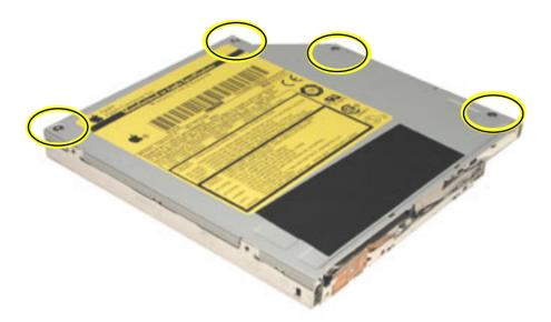
2. Slide the top cover approximately 2 mm toward the back of the drive. Lift up the top cover to remove it.
