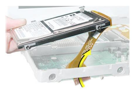
7. Disconnect the hard drive bracket (with grommets attached) by pulling it straight off the drive.
