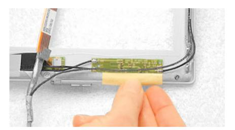
3. Warning: When lifting the antenna board, be careful not to strain or pinch the cables.
