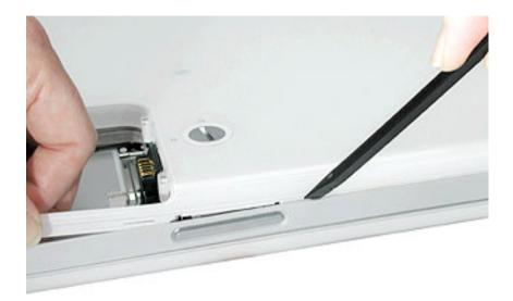
10. Warning: To avoid damaging the sleep light and other delicate components, do not insert the black stick too far into the computer as you free the bottom case from the computer. Use just the tip of the black stick to pry up the bottom case.
