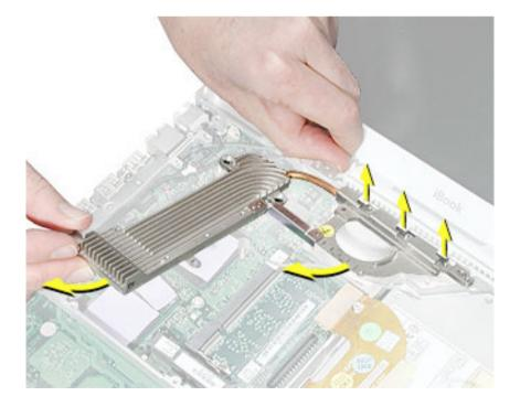
5. Turn over the heatsink and note the L-shaped marks that indicate the position for placement of the thermal pads.
