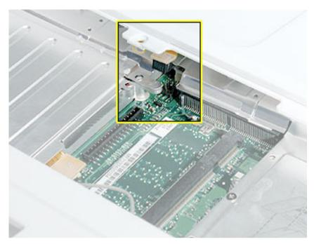
**Replacement Note:** When the top case is removed, the trackpad cable automatically disconnects from the logic board. However, when installing the top case, use a black stick to press down on the connector, and make sure the trackpad cable connects securely to the four pins on the logic board.
