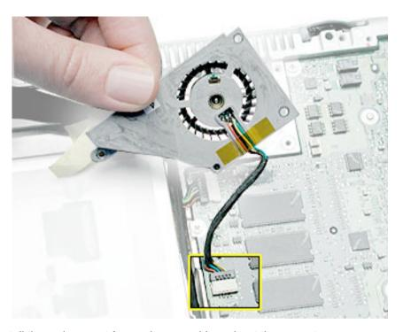
4. Install the replacement fan, and reassemble and test the computer.
