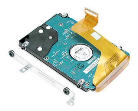
8. Warning: Handle the hard drive at the sides only. Do not touch or press anywhere else on the drive.
