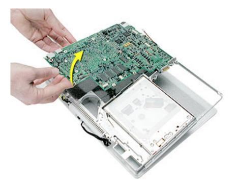
6. Install the replacement logic board, and reassemble and test the computer.
