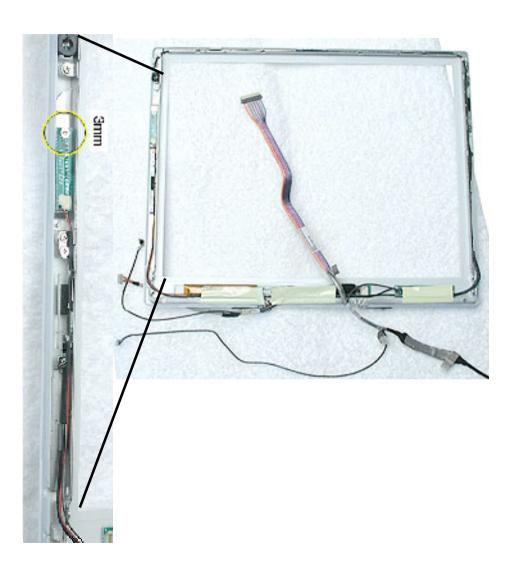
3. Lift up the cables and peel up the tape that covers the cables running along the bottom of the inverter board.
