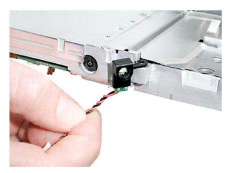
5. Install the replacement sleep light board, and reassemble and test the computer.
