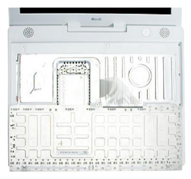
**Note:** If no replacement AirPort Extreme Card is to be installed, the antenna cable should be routed as shown.
