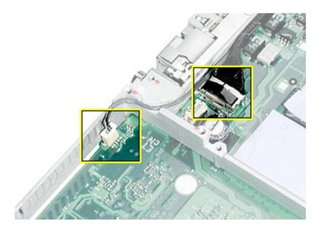
2. Disconnect the optical drive flex cable.
