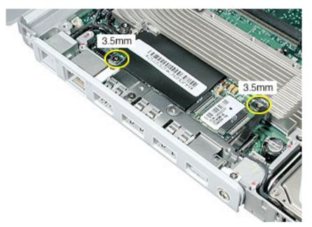
3. Disconnect the cable from the upper end of the modem board.
