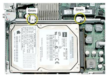
5. From the bracket side, tilt up the hard drive, and hold it by the sides of the drive.
