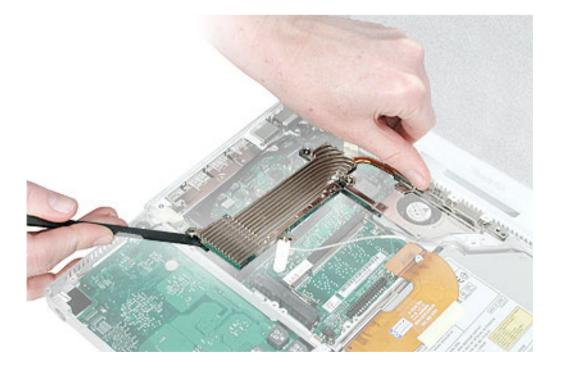
5. Turn over the heatsink and note the position of the thermal pads.
