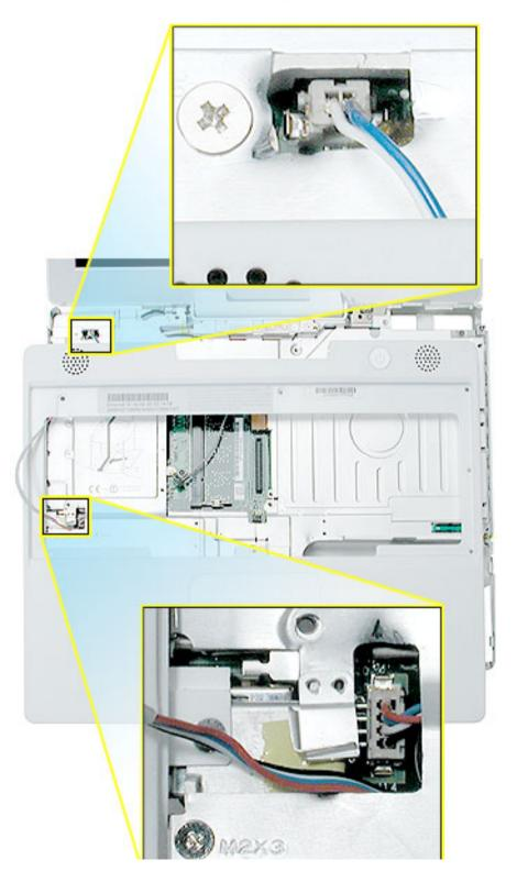
**Replacement Note:** When connecting the speaker cable, make sure the wires are routed under the top shield as shown.
