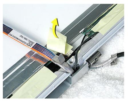
13. Warning: When lifting the LCD panel, be careful not to strain the inverter cable.
