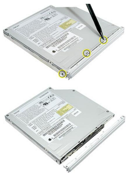
12. Install the replacement optical drive, and reassemble and test the computer.
