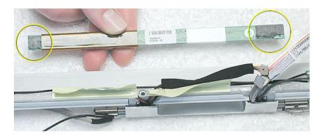
4. Install the replacement inverter board, and reassemble and test the computer.
