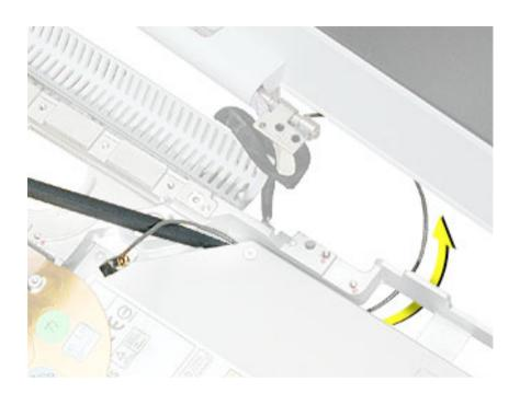
9. Remove the display from the computer chassis.
