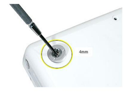
6. Remove the two identical Phillips screws next to the battery connector.
