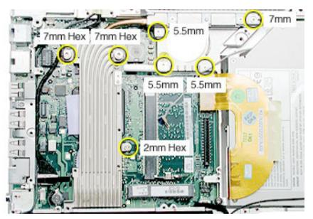
**Replacement Note:** When installing the heatsink, install the screws in the order shown.
