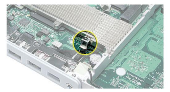
2. Remove the two screws from the vent cover and tilt up the vent cover slightly.
