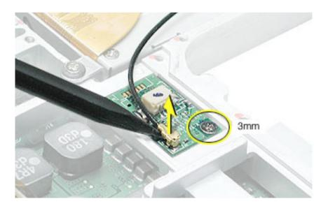
4. Without putting pressure on the optical drive, support the antenna board holder in place as you slide out the antenna board.
