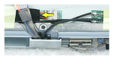
6. Remove the reed switch cable assembly.
