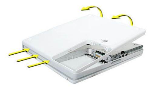
14. If you are replacing any additional parts at this time, remove the two springs from the battery compartment so they do not fall out and get lost.
