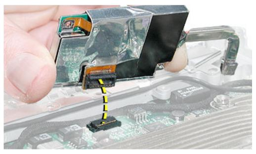
**Replacement Caution:** Handle the modem by the edges only. When securing the modem to the logic board, press only on the rectangular area (highlighted in green in the following image) that is directly over the modem connector.
