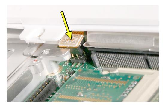
10. Place the computer on its side, and with most of the top case loosened, tilt the top case away from the computer latch.
