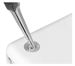
6. Use a screwdriver to remove the screw and socket from the bottom case.
