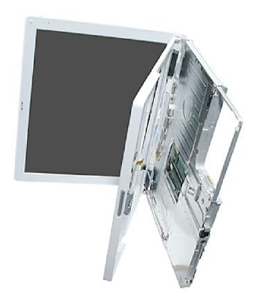
12. Place the computer upright, and move the top case off center. Use a black stick to carefully disconnect the two cables from the logic board.
