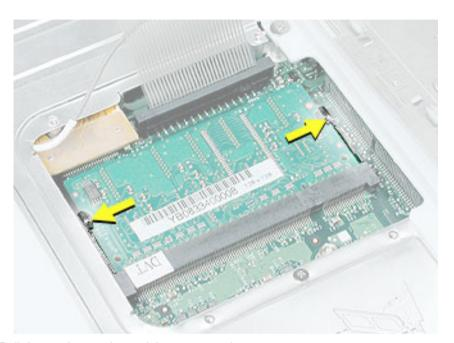
3. Pull the card up and out of the memory slot.
