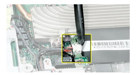
4. Tilt up the modem and metal shield to remove them from the computer.
