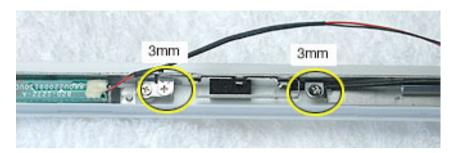
9. Tilt up the antenna receptor to remove it from the left side of the bezel assembly.
