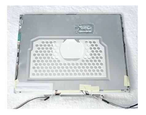
5. Peel up the tape if it covers the two screws at the clutch. Remove the two Phillips screws.
