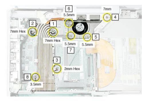
**Replacement Note:** When installing the 3.5-mm long screw and EMI clip at the lower left end of the thermal plate, make sure the EMI clip is installed as shown.
