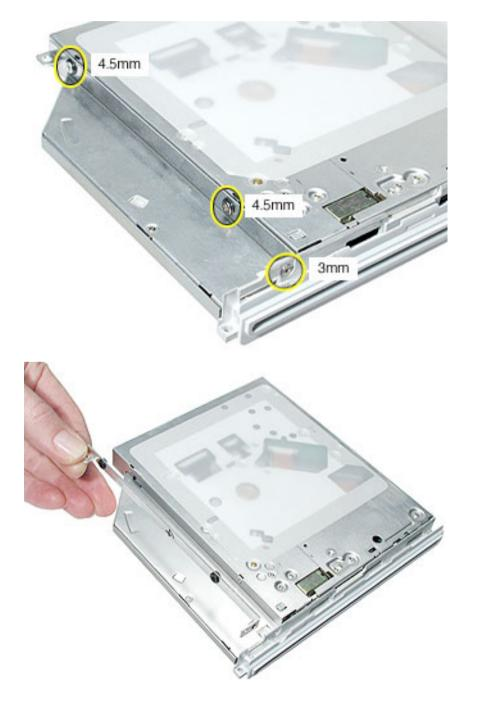
11. **Caution:** The bezel and optical drive case is a soft material. Be especially careful when removing the bezel from the optical drive.
