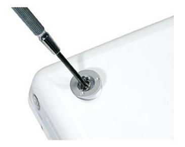
7. Install the new socket. For the best fit, do not reuse the old socket.
