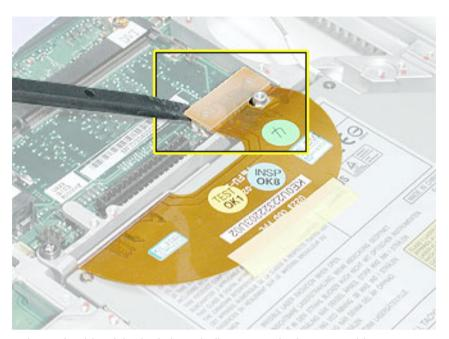
3. From the underside of the logic board, disconnect the inverter cable.
