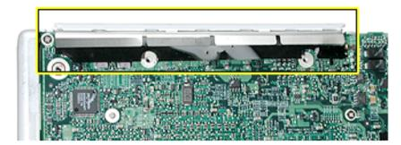
**Replacement Note:** Note the placement of the long EMI strip that covers the FireWire port, USB ports, and display port. Make sure it is held in place by the single screw before reassembling the computer.
