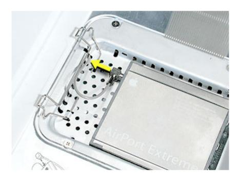
4. Use the pull-tab on the card to remove the card from the slot.
