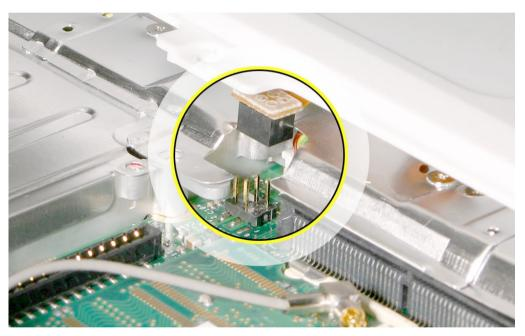
Warning: When reassembling the computer, be careful not to pinch any cables as you press the top case back onto the computer. Check that the top case shows no raised surfaces and is fully snapped into place before installing the remaining screws.
