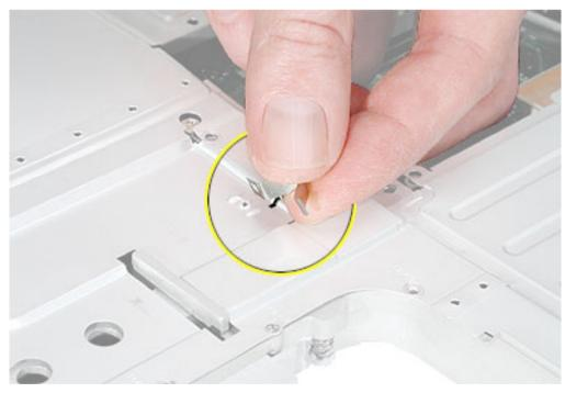
**Replacement Note:** Before installing the top shield, make sure cables are routed as shown, and fresh tape is installed where shown.
