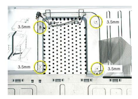
**Replacement Note:** Note the routing of the AirPort antenna cable. When reinstalling the RAM shield, make sure the antenna cable is routed as shown if there is no AirPort Extreme Card.
