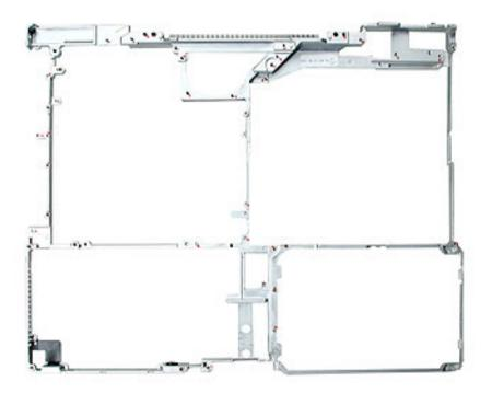
**Replacement Note:** The front of the frame includes two integral grommets for positioning the hard drive. Make sure the grommets are in place before reassembling the computer.
