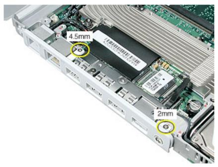
2. Remove the I/O bezel from the computer frame.
