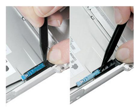
5. **Note:** If the antenna board holder is attached securely, you do not need to replace it when installing a replacement Bluetooth antenna board. However, if you are replacing the optical drive with a new drive, remove the antenna board holder and install a new one on the replacement optical drive. The antenna board holder adheres to the optical drive with an adhesive backing.
