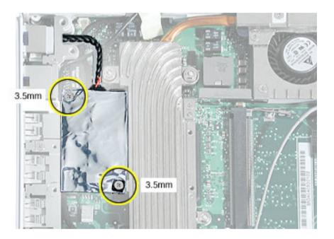
3. Carefully grasping the ends of the modem board and shield, lift them straight up to disconnect them from the logic board.
