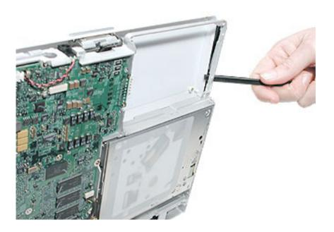
9. As you begin to loosen the top case, check that the trackpad cable (orange flex cable) has disconnected from the top case. Or use a black stick to disconnect it.
