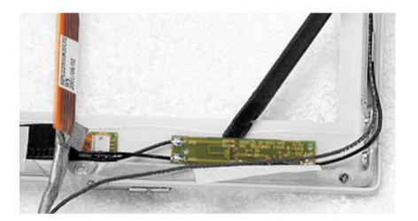
4. With the antenna board loosened, note the cable routing on each side of the bezel. On the right, the antenna receptor cable is routed underneath the microphone cable through two channels before terminating at the receptor bracket.
