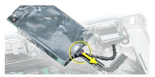
5. Install the replacement modem, and reassemble and test the computer.
