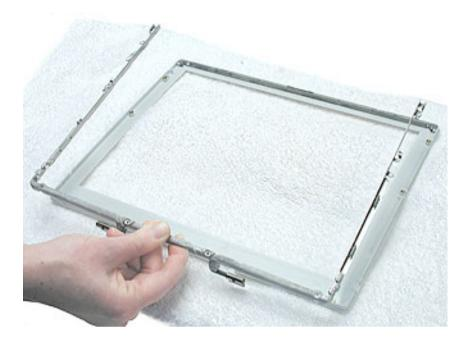
6. Install the replacement bezel brace with clutch assembly, and reassemble and test the computer.
