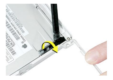
6. Install the replacement Bluetooth board and antenna, and reassemble and test the computer.
