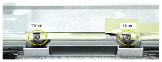
6. Tilt up the display assembly and pull straight down on the display clutch cover.
