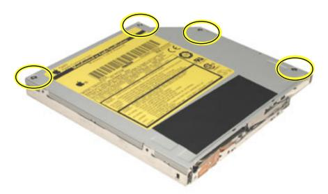
2. Slide the top cover approximately 2 mm toward the back of the drive. Lift up the top cover to remove it.
