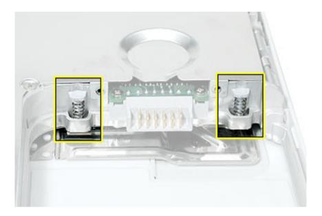
**Note:** When reassembling the computer, make sure that the two springs in the battery compartment are in place before installing the bottom case. Each spring has a plastic cap on one end. The cap should fit securely on the spring, and the curved side of the cap should be positioned against the inner frame. The springs have a small amount of grease on them; do not wipe away the grease.
