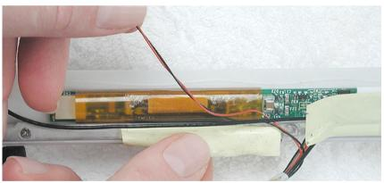
4. Warning: When removing the tape that bundles the reed switch cable assembly to the AirPort Extreme Card antenna cable, be careful not to strain or pinch the cables.
