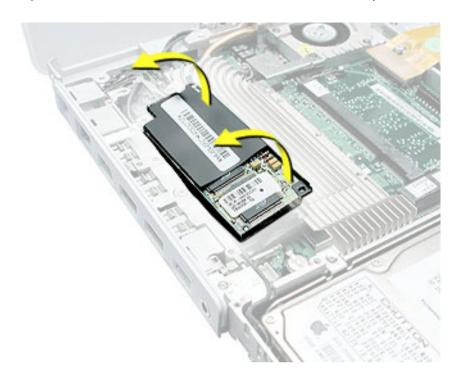
Install the replacement modem, and reassemble and test the computer.
