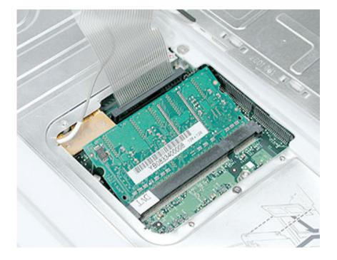
4. Align the notch in the replacement memory card with the small tab in the memory slot. Hold the card at a 30-degree angle, then push the card into the slot until it is firmly seated.
