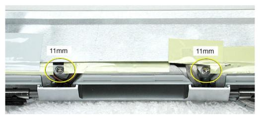
9. Peel up the tape that anchors the folded mesh strip of the LCD cable to the shield.
