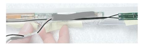
8. On the left side of the bezel, remove the two Phillips screws at the antenna receptor.
