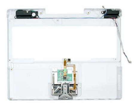
**Important:** Make sure you transfer the original serial number label and Ethernet label from the old top case to the replacement top case. You can use a black stick to carefully peel up a corner of the label. Then peel off the label completely and apply it to the replacement top case. Make sure that the labels lie completely flat so they do not interfere with the battery compartment.
