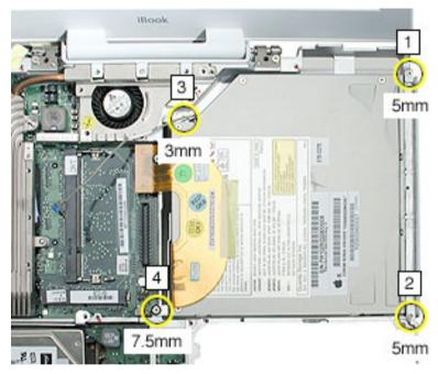
4. Disconnect the optical drive ribbon cable from the logic board.
