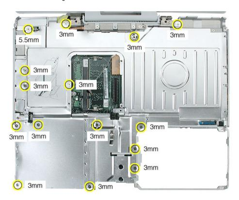
Replacement Note: When replacing the shield, install the screws in the order shown.
