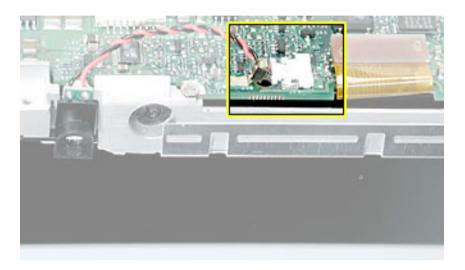
3. Turn over the computer and remove the single screw from the sleep light holder and frame.
