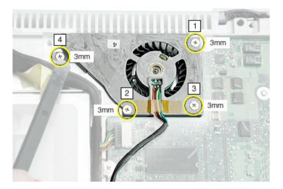
3. Lift the fan from the computer, and use a black stick to disconnect the connector from the logic board.
