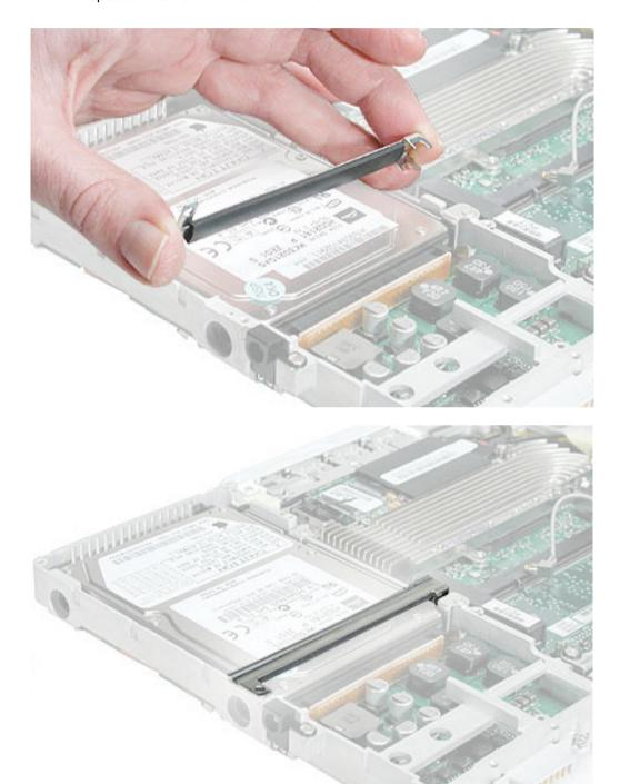
**Important:** If you are installing the same top shield, remove the EMI finger by twisting it off of the shield. If you are replacing the top shield, make sure the shield does not have the EMI finger attached. A new foam pad on the trackpad overrides the need for the EMI finger.
