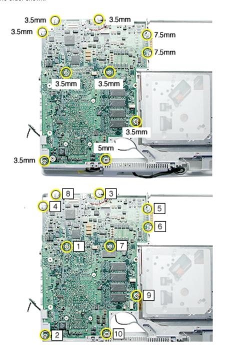
5. **Warning:** Flexing the logic board can break solder joints to components. To prevent damage, do not flex the board.
