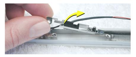
10. Unwrap the tape that secures the AirPort Extreme Card antenna to the cable bundle.
