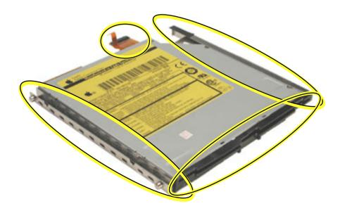
1. Remove the four identical screws that hold the top cover to the drive.
