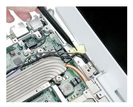
6. While supporting the display, tilt up the chassis, and disconnect the inverter cable from the underside of the logic board.
