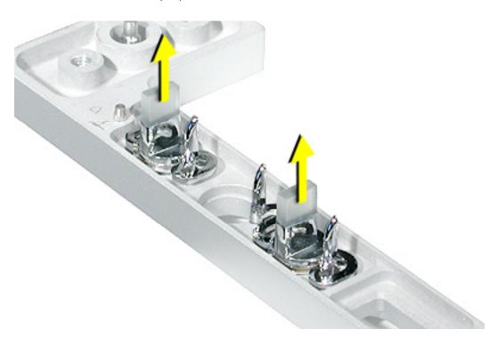
**Replacement Note:** Position the replacement buttons in the front bezel as illustrated.
