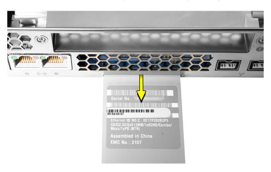
2. Gently grasp the ID tab and pull up on it to disengage it from the channel that it slides along in the enclosure.
