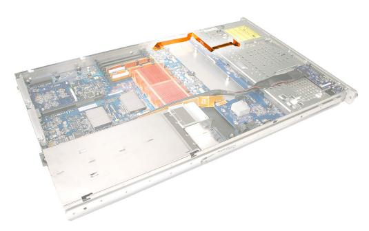
Warning: The optical drive cable is attached to the enclosure with adhesive on the underside of the cable.
