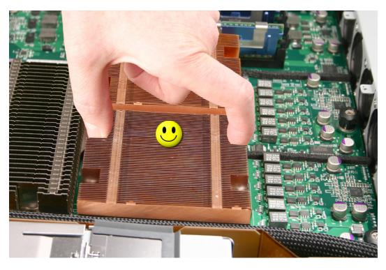
2. Caution: Each heat sink is connected to the logic board by a small 2-pin thermal sensor cable. Lifting the heat sink too quickly can damage the cable or connector. Because of the tight thermal bond between the processor and heat sink, be especially cautious to initially lift the heat sink no more than one centimeter (1 cm) off the processor. Do not pull on the cable as you lift the heat sink enough to disconnect the cable from the logic board.
