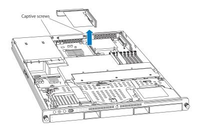
3. Tilt the expansion card up so that its port clears the enclosure, and remove the card from the Xserve.
