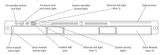
Note: The front bezel of the Xserve (Early 2008) model is identical to the Xserve (Late 2006) image above except the FireWire 400 port is replaced by a USB port, as shown below:
