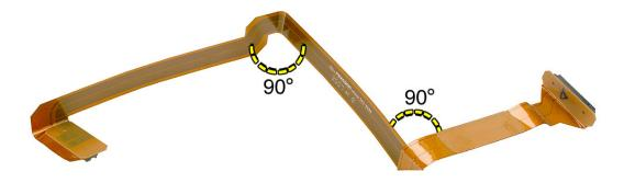
Replacement Note: Connect the replacement optical drive cable to the logic board first. Then press the adhesive section of the cable onto the enclosure before connecting the other end of the cable to the optical drive.
