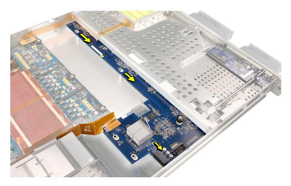
5. Rotate the backplane up slightly from the logic board side (as shown), and carefully pull the backplane up and toward the logic board to free it from the standoffs and four backplane alignment slots in the enclosure. Be careful not to let any backplane components come into contact with the standoffs or the enclosure as you remove the backplane.
