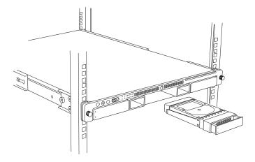
Replacement Note: Press and release the handle on the replacement drive to open it, and slide the module into the bay until it is firmly seated. Then press the handle in flush with the front panel. The disk status light will turn green to indicate normal operation.
