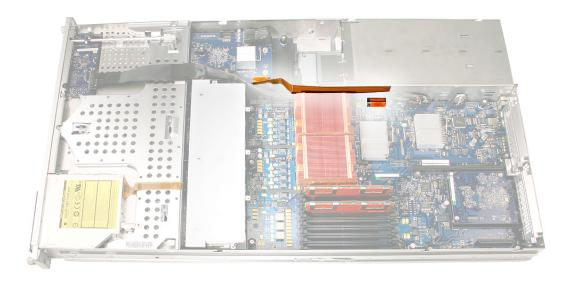
Disconnect the backplane-to-logic board cable from the logic board.
