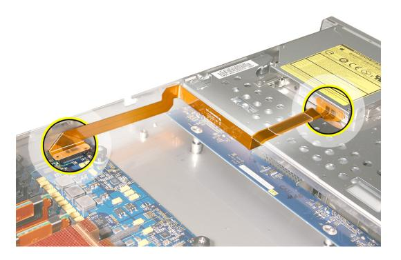
Carefully pry the cable's adhesive from the enclosure and remove the cable from the Xserve.
