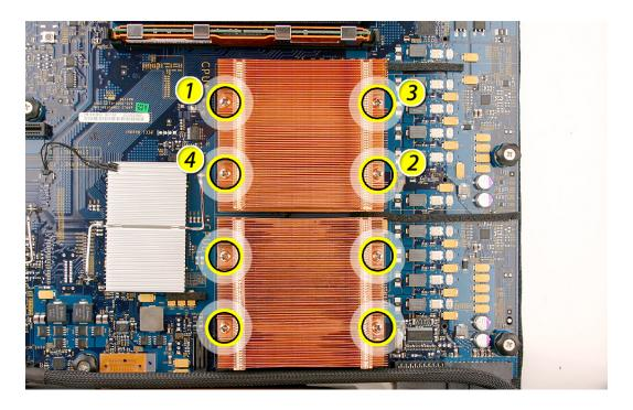
Caution: Whenever you handle the heat sink, handle it from the slotted sides, not the smooth sides. Grasping the smooth sides of the heat sink can compress its ribs causing permanent damage.
