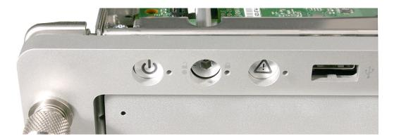
Replace the bezel brackets, four 4-mm long screws, and 8-mm long center screw with star washer.
