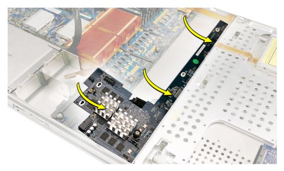
Then rotate the Xserve RAID Card downward and over the four mushroom-shaped standoffs. Finally, slide the card in the direction of the arrow shown to fully seat the card in the enclosure.
