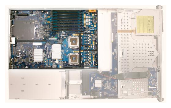
Caution: Although the logic boards for Xserve (Late 2006) and Xserve (Early 2008) are a similar size, do not install an older logic board in the Xserve (Early 2008) server.
