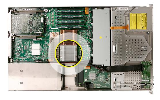
1. Loosen the four screws securing the heat sink that is closest to the DIMM slots (CPU A) in the order indicated below.
