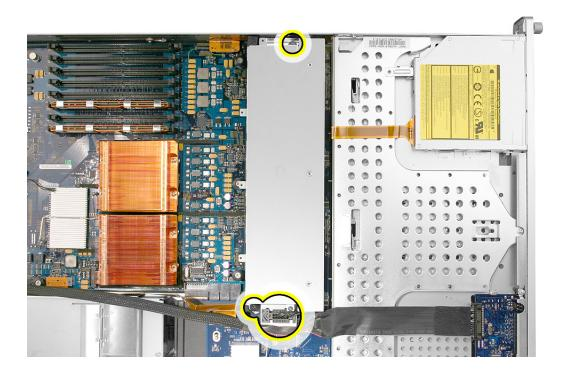
Replacement Note: Push down on the fan array power connector to seat it when installing the fan array.
