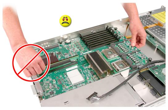
Caution: When transferring the logic board, be careful not to flex the logic board, which could damage the board or its components. To best distribute the weight of the logic board and minimize flexing, hold the logic board at the long sides near the center, as shown.
