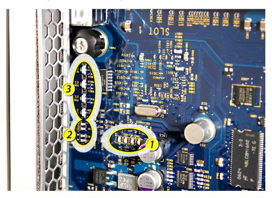
The LEDs are located toward the rear of the logic board. You must remove the top cover of the Xserve for the diagnostic LEDs to function.
