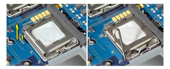
3. Carefully lift the processor out of the holder.
