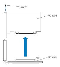
WARNING: When removing or installing an expansion card, handle it only by the edges. Do not touch its connectors or any of the components on the card. Lift the card straight out from the connector to remove it, and insert it straight into the connector to install it. Do not rock the card from side to side and don't force the card into the slot. Once the replacement card is installed, pull on it gently to check that it is properly connected.
