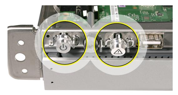
2. Make sure the light pipe is secure in the front bezel. If it comes out, align the pins to the front bezel, and insert it into the slot in the front bezel.
