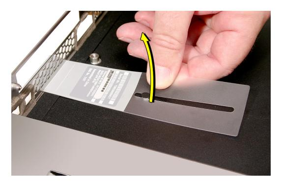
Pull the ID tab through the slot in the rear panel to remove it.
