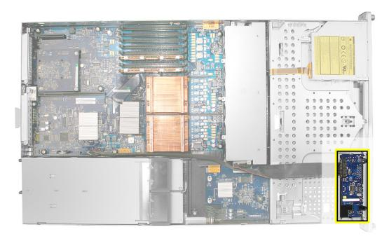
Release the two locking levers on the front panel board cable connector and disconnect the cable from the front panel board.
