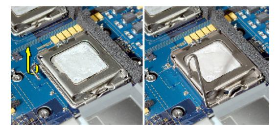
3. Carefully lift the processor out of the holder.
