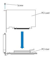
3. If you are removing a riser card so that you can replace it with a new riser card, remove any expansion card installed in the original riser card and transfer the card to the replacement riser.
