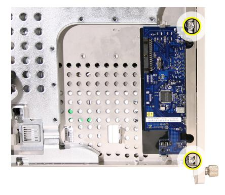
3. Slide the board back slightly and release the two clips on either side of it.
