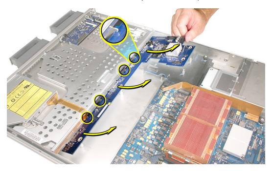
Replacement Note: When installing the backplane, lower the backplane into the enclosure at a slight angle (as shown), and carefully align the front edge of the backplane with the four backplane alignment slots in the enclosure. Be careful not to let any backplane components come into contact with the standoffs or the enclosure as you install the backplane.
