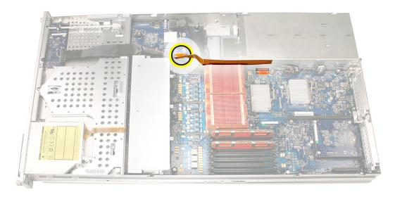
**Replacement Note:** Before installing the cable, fold it to a 90-degree angle along its creases.
