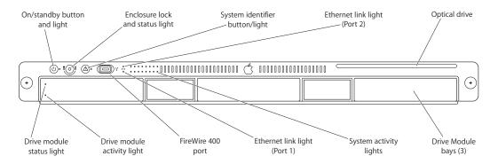
Note: The front bezel of the Xserve (Early 2008) model is identical to the Xserve (Late 2006) image above except the FireWire 400 port is replaced by a USB port, as shown below:
