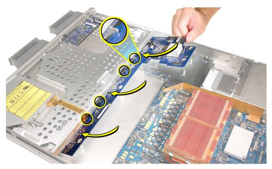
Then rotate the backplane downward and over the four mushroom-shaped standoffs. Finally, slide the backplane in the direction of the arrow shown to fully seat the backplane in the enclosure.
