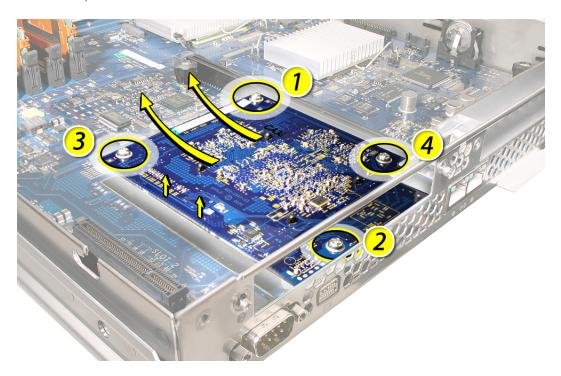
Replacement Note: When installing the mezzanine card, be sure to press down gently and evenly on it to seat the connector on the underside of the card to the logic board. Then replace the four screws, and secure them in the order shown above.
