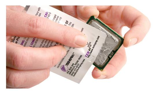
Holding the processor by three corners only, keep the processor level as you place it into its holder on the logic board, being careful not to get any thermal grease on the contacts of either the processor or its socket holder.
