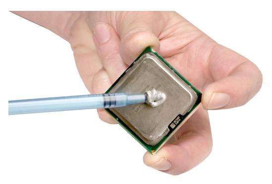
6. Use the edge of the package that the alcohol wipe came in as a spatula to spread the thermal grease evenly over the entire top surface of the processor. Scrape off any excess grease with the package edge, then discard the package.
