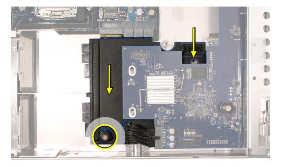
Note: Don't remove the power distribution board but make sure its edge connector is all the way out of the connector on the logic board.
