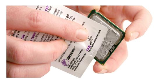
3. Holding the processor by three corners only, keep the processor level as you place it into its holder on the logic board, being careful not to get any thermal grease on the contacts of either the processor or its socket holder.
