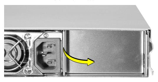
2. Notice the hook that catches on the inside bottom of the power supply bay.
