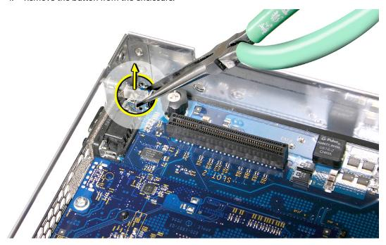
Replacement Note: When installing the rear ID button, take care not to bend or break the four small plastic prongs as you work the button back through the opening in the rear enclosure. Make sure all four prongs are properly seated in their respective holes in the logic board.
