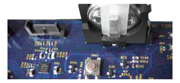
**Note:** After installing a replacement logic board, be sure to transfer the processors, heat sinks, video mezzanine board, any expansion cards, PCI riser cards, and FB-DIMMs to the new board. You must also remove the battery insulator tab from the battery holder on the new board.
