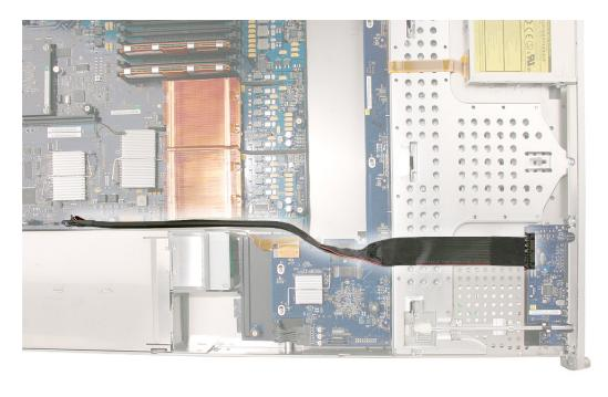
Release the locking levers on the cable connectors and disconnect the front panel board cable from the front panel board and the logic board.
