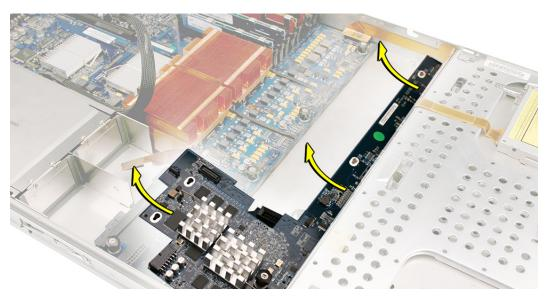
Replacement Note: When installing the Xserve RAID Card, lower the card into the enclosure at a slight angle (as shown), and carefully align the front edge of the card with the four alignment slots in the enclosure. Be careful not to let any Xserve RAID Card components come into contact with the standoffs or the enclosure as you install the card.
