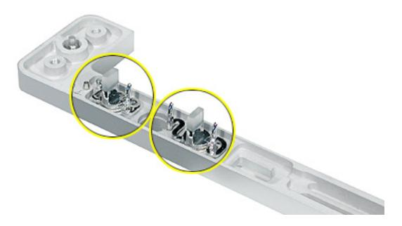
2. Position the light pipes in the light pipe assembly into the double row of light pipe holes in the front bezel.
