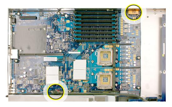
4. Loosen the single thumbscrew on the power distribution board and slide the board away from and out of the connector on the logic board.
