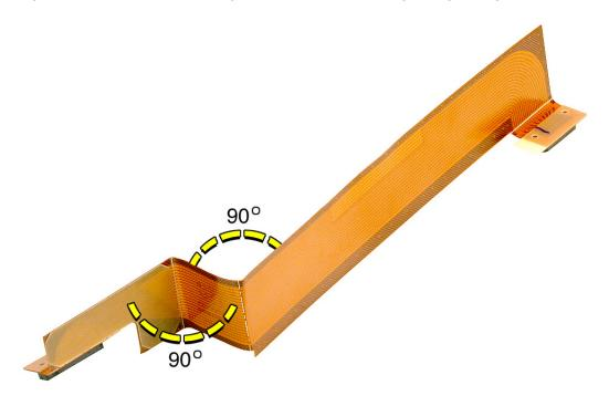
Replacement Note: Connect the cable to the logic board first. Then press the adhesive section of the cable onto the enclosure before connecting the other end of the cable to the backplane.
