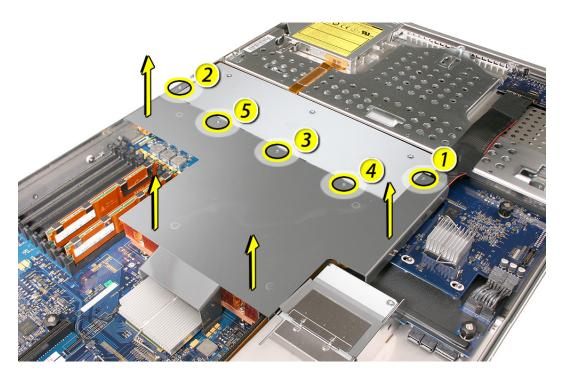
Caution: Try not to completely remove the screws from the airflow duct. Tiny black rubber washers hold these screws captive on the underside of the airflow duct. If the screws are completely removed, these rubber washers can easily fall into the enclosure and become lost.
