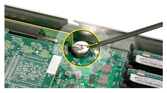
2. Insert the replacement battery in the holder with the positive side (+) up and the negative side down.
