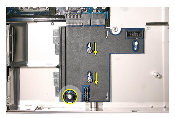
3. Lift up the board and remove it from the enclosure.
