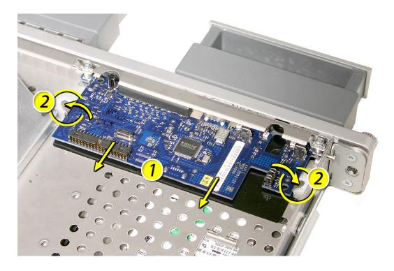
4. Tilt the board up and remove it from the Xserve.
