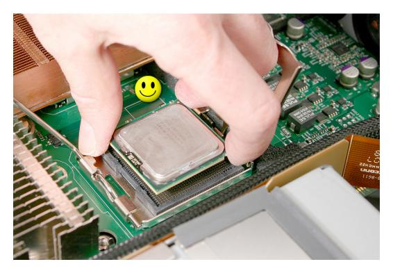
Note: When installing the processor on the logic board, align the processor notch with the tab on the processor holder, as shown. Then lower the processor straight down onto the socket.
