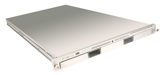
The only noticeable external difference between the Xserve (Late 2006) model and the Xserve (Early 2008) model is the port next to the system identifier button on the front bezel. On the Xserve (Late 2006) model, it is a FireWire 400 port; whereas on the Xserve (Early 2008) model, it is a USB port, as shown below.
