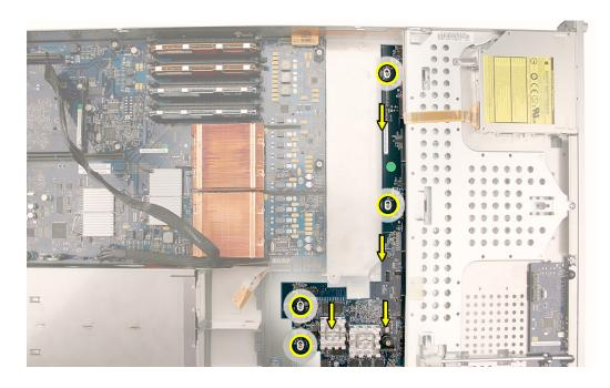
6. Rotate the Xserve RAID Card up slightly from the logic board side (as shown), and carefully pull the card up and toward the logic board to free it from the standoffs and four alignment slots in the enclosure. Be careful not to let any Xserve RAID Card components come into contact with the standoffs or the enclosure as you remove the card.
