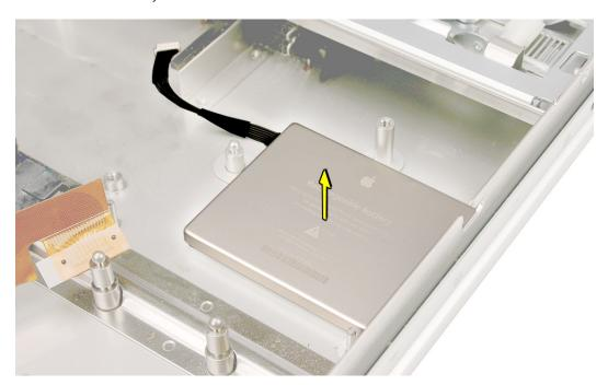
Replacement Note: Before installing a new battery, remove the protective film covering the adhesive on the underside of the battery. Then lower the battery into place on its three mounting posts.
