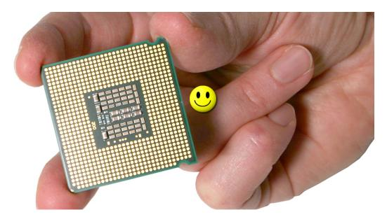
4. Clean off any existing thermal grease on the top face of the processor using the alcohol wipe provided with the replacement part, being careful not to get any thermal grease on the processor contacts.
