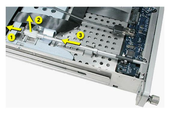
3. If you are replacing the plastic gear on the end of the rod, slide the gear off the rod.
