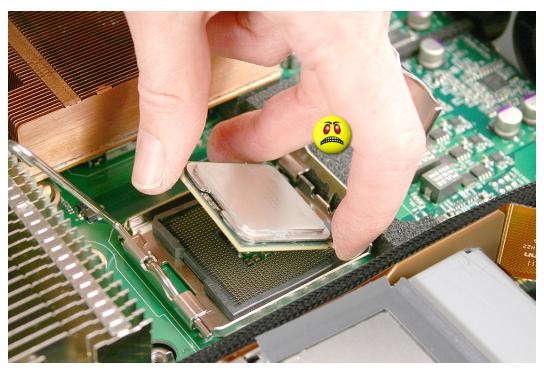
**Note:** When installing the processor on the logic board, align the processor notch with the tab on the processor holder, as shown. Then lower the processor straight down onto the socket.
