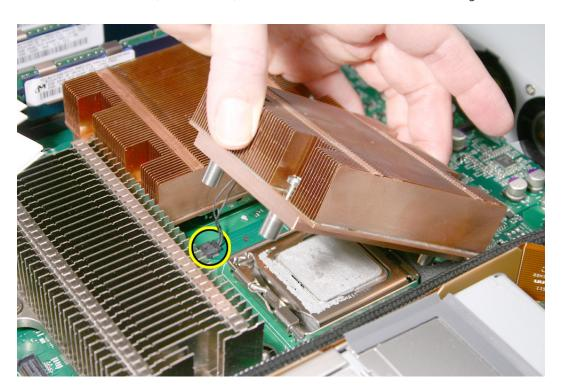
4. Lift the heat sink straight up and out of the enclosure.
