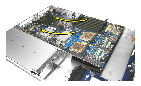
Replacement Note: Remove the battery insulator tab from the battery holder on the replacement logic board. Depending on the Xserve model, the battery position may differ from what is shown.
