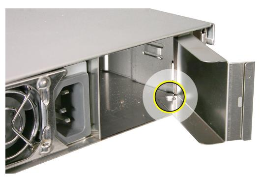
3. Open the power supply blank as far as it will go, and then pull out the power supply blank.
