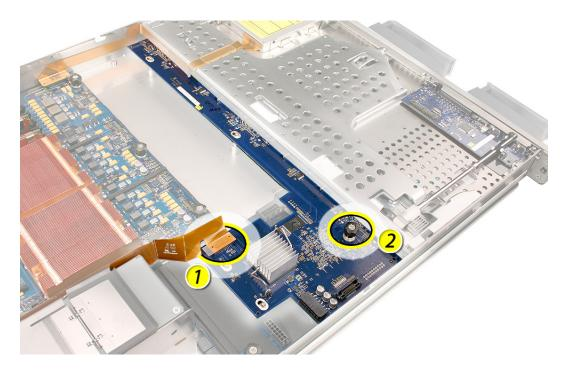
4. Shift the backplane to the left (towards the enclosure side), in the direction of the arrow shown, until it clears the four mushroom-shaped standoffs that hold the backplane in place.
