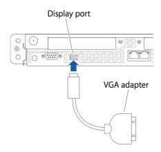
A mini-DVI to VGA display adapter (such as the one shown above) is included with the Xserve. The Xserve mini-DVI display port also supports other optional Apple video adapters, such as the Apple mini-DVI to DVI adapter, and the Apple mini-DVI to Video adapter.
