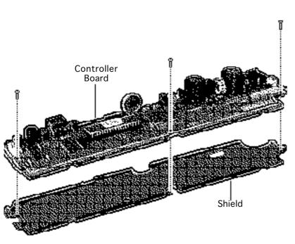
2 Using a small Phillips screwdriver, remove the three screws and remove the controller board from the shield.
