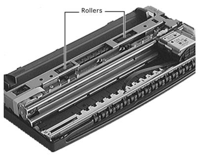
Using a dry cloth, carefully wipe the rollers.
