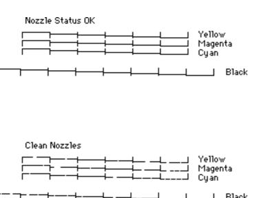
Examine the bottom of the test page to determine print head status.
