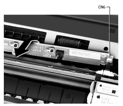
Tilt the board up, and gently remove the ribbon cable from connector CN6.
