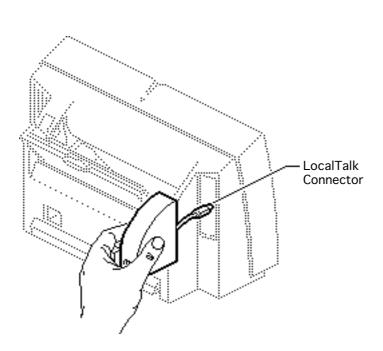
2 Plug the LocalTalk connector into the serial port.
