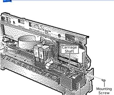
7 Using a Phillips screwdriver, remove the mounting screw from the carriage shaft.
