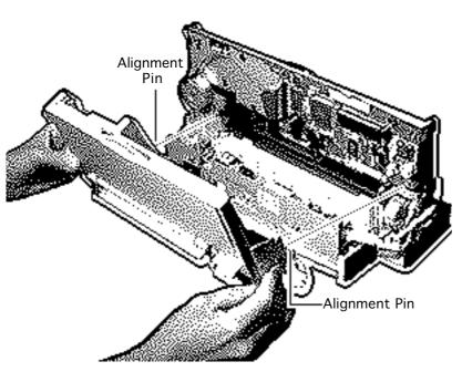
Replacement Note: Make sure the alignment pins on the cut sheet feeder are aligned with the printer frame.
