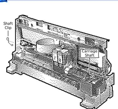
8 Carefully remove the shaft clip from the carriage shaft.
