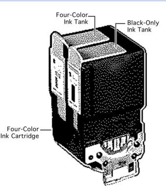
**Note:** This procedure covers ink tank replacement for the four-color ink cartridge. The cartridge contains two separate ink tanks, one for black ink and one for cyan, magenta, and yellow inks. When you run out of ink, you replace only the empty tank, instead of replacing the entire cartridge.
