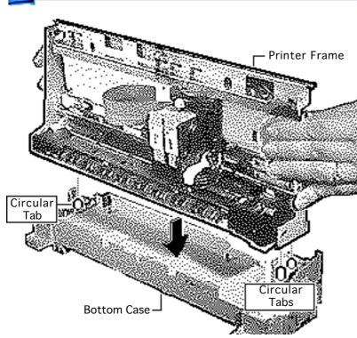
Replacement Note: Make sure the bottom case circular tabs fit into the proper position in the printer frame.
