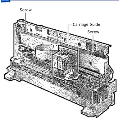
Caution: Do not remove or loosen the two screws on top of the carriage guide.
