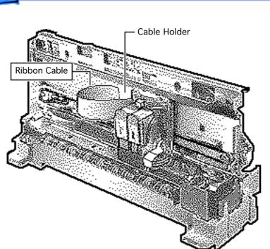
4 Remove the plastic ribbon cable and cable holder from the printer.
