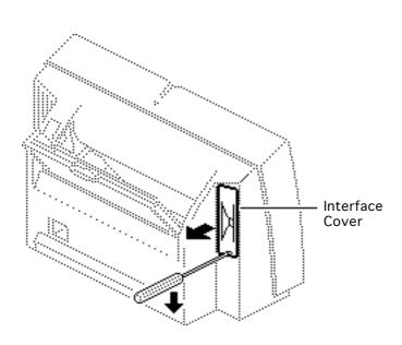
1 Using a small flat-blade screwdriver, release the mounting tab and remove the interface cover from the rear case.
