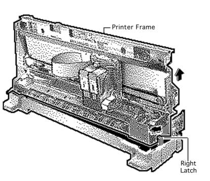
**Note:** The printer frame is not a replaceable part. Remove the frame to access the purge unit, paper feed motor, ink absorbers, and bottom case.
