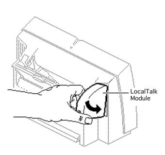
3 Insert the upper edge of the LocalTalk module into the rear case, and then snap the bottom into place.
