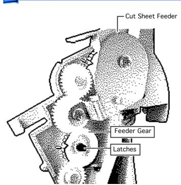
1 Caution: When the roller is removed, the feeder gear is loose. Remove the roller slowly so that the gear will not fly off.
