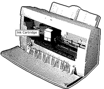
**Note:** This procedure covers the ink cartridge replacement for either of the ink cartridges that come with the printer. One cartridge is black ink only; the other is a four-color ink cartridge with two ink tanks. One tank contains black ink only and the other tank contains the cyan, magenta, and yellow inks.
