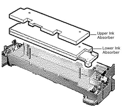
If the ink absorbers have been used for two weeks or less, or if fewer than 50 pages have been printed, it is not necessary to replace the ink absorbers when replacing the logic board.
