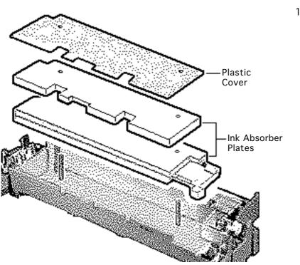
Remove the clear plastic cover and the two ink absorber plates.
