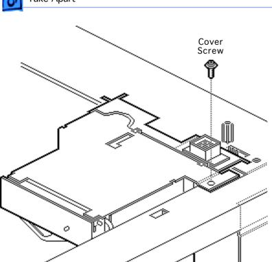
Remove the single black screw that secures the controller block cover.
