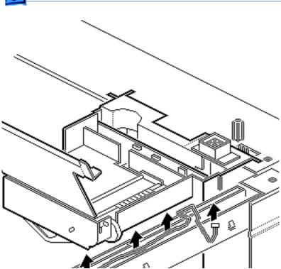
4 Remove the cables from the channel in the right frame.
