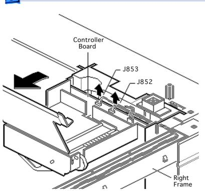
3 Cut the cable tie (if present) and disconnect the two cables that run across the right frame to the drive block.
