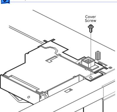
Remove the single black screw that secures the controller cover.
