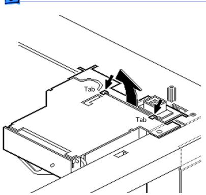
2 Release the two flex tabs and swing the cover upward.
