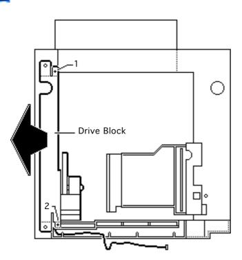
Remove the two screws and lift the drive block out of the sheet feeder.
