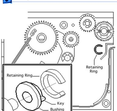
Replacement Note: The bushing is plastic and is keyed. When properly installed, the bushing nests within the Cshaped retaining ring in the drive block. When installing the motor assembly, make sure that the key is pointing to the right, toward the open end of the C.
