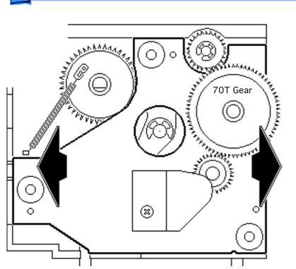
3 Remove the motor assembly from the drive block.
