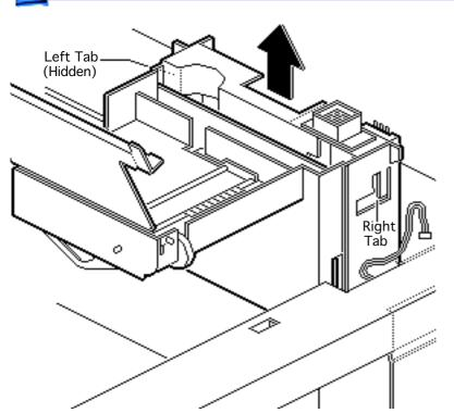
5 Release the two flex tabs and slide the block up and out of the feeder.
