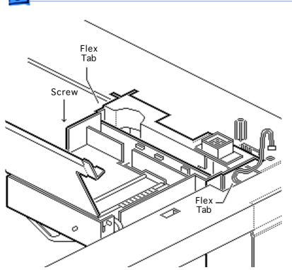
4 **Note:** One screw and two flex tabs attach the controller block to the feeder. The flex tabs are located on the sides of the block about an inch from the top surface.
