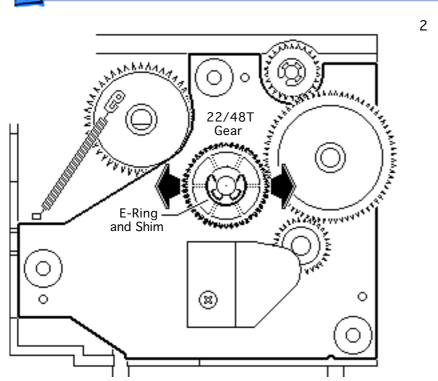
2 Remove the E-ring and the shim washer and pull off the 22/48T gear.
