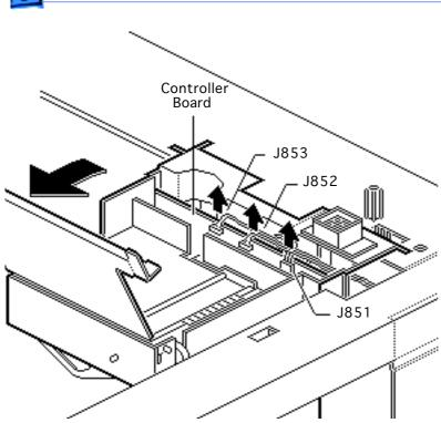
3 Cut the cable tie (if present) and disconnect the three cables from the controller board.
