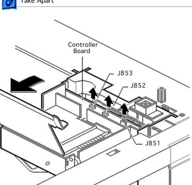
Cut the cable tie (if present) and disconnect the three cables from the controller board.
