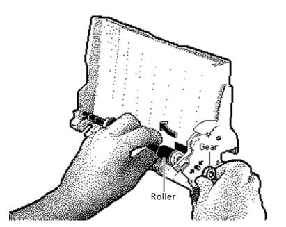
1 **Caution:** When the roller is removed, the feeder gear is loose. Remove the roller slowly so that the gear will not fly off.
