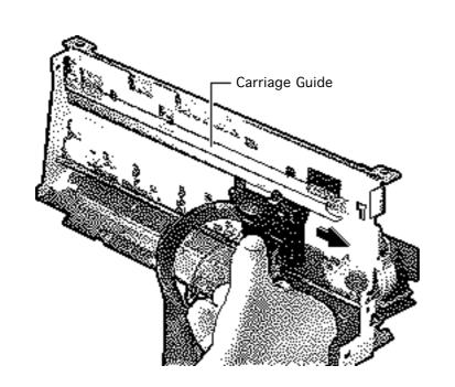
6 Move the carriage to the far right and disconnect the carriage from the carriage guide.
