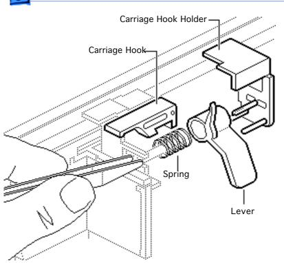
Replacement Note: To reassemble, put the cartridge hook on its post on the cartridge carrier, and put the blue lever and spring over the central post of the holder. Slide the assembly into place as you mesh the ridge on the lever with the groove on the bottom of the cartridge hook. Snap the assembly securely into place.
