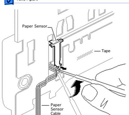
1 **Note:** The paper sensor cable is attached to the back of the printer frame with double-stick tape.
