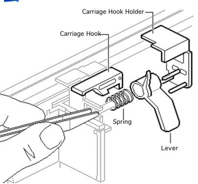
4 **Note:** The four pieces of the cartridge hook assembly (the holder, spring, lever, and hook) will fall into your hand when you perform this step.
