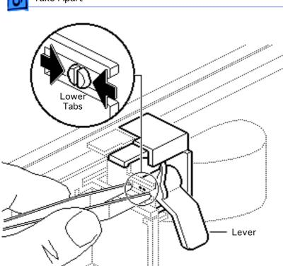
3 Using small needlenose tweezers, gently squeeze the tips of the lower tabs inward and release the spring that holds the lever in position.
