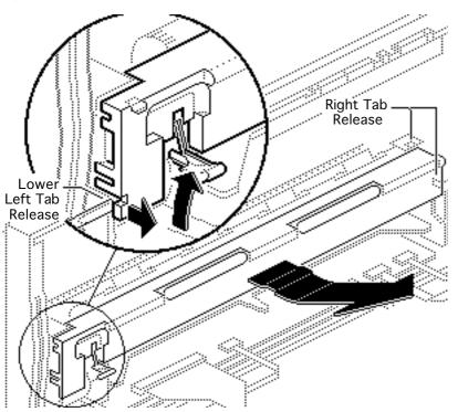
screwdriver, gently pry between the platen cover and printer frame and free the lower left tab release.
