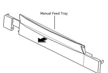
7 Remove the manual feed tray by flexing it enough to free the plastic hinges from the lower access cover.
