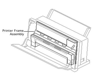
Caution: You must replace Revision A and Revision B printer frame assemblies like-for-like. If you are replacing the frame assembly, see "Revision Identification" in Additional Procedures.
