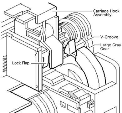
necessary to push gently on the carriage hook assembly or to rotate the worm screw slightly to slide the carriage hook assembly.
