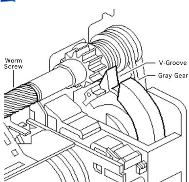
2 Rotate the carriage worm screw until the Vgroove of the large gray gear faces up.
