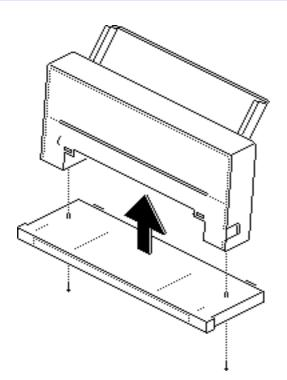
Remove the two screws and lift off the output tray and base assembly.
