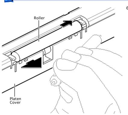
Note: It is not necessary to remove the platen cover from the printer frame to remove a roller.
