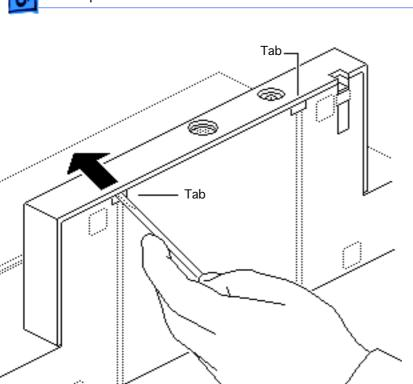
1 Using a small flat-blade screwdriver, gently pry up and release the two tabs on the bottom of the printer.
