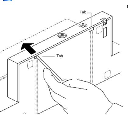
1 Using a small flat-blade screwdriver, gently pry up and release the two tabs on the bottom of the printer.
