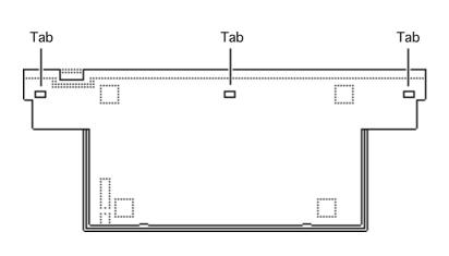
Caution: Be careful not to bend or break any of the plastic tabs on the StyleWriter. Use jeweler's screwdrivers and precision tweezers and do not apply excessive force.
