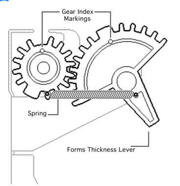
Note: The forms thickness lever kit contains the forms thickness lever and its spring.
