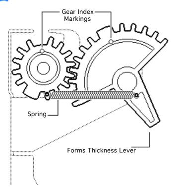
Replacement Note: The forms thickness lever is actually a gear that meshes with a second gear behind it. The second gear attaches to the carriage shaft that controls the distance of the ink cartridge from the paper. Note the gear index markings that align when the gears are in the middle of the range. Align these markings during reassembly.
