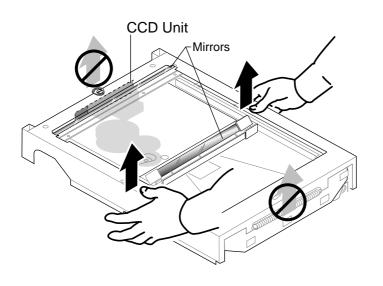
Hold or lift the optical assembly by the long sides, never by the shorter sides.
