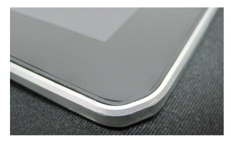
Corner dent resulting in multiple cracks:
