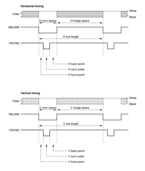
To accommodate the various VGA and SVGA modes on the Macintosh monitors, the video controller must have its timing parameters changed by the BIOS. To do that, the Macintosh software reads the video sense lines and loads the appropriate values for the video BIOS before starting up the PC. (Remember that system and video BIOS reside in Macintosh system memory and are modifiable by the software.)
