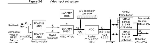
The input signal, which may be analog composite or S-video in NTSC, PAL, or SECAM format, enters through an external 7-pin mini-DIN socket. A cable adapter is provided to receive composite video from external devices that have RCA connectors. TDA8708 and TDA8709 video ADC chips digitize the composite video waveform, and the DMSD chip decodes the result into YUV format. This common digital video format, also known as YCrCb, is described in CCIR Recommended Standard 601-2.
