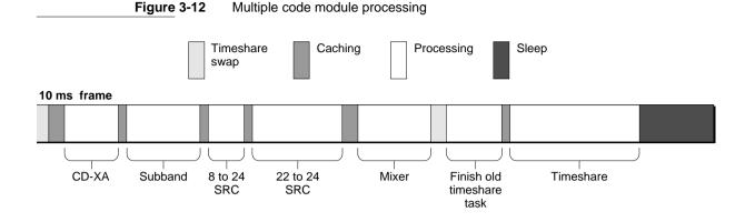
As Figure 3-12 shows, the five required real-time processing modules are run in sequence. The timeshare algorithm that was running when the frame started is reloaded and completed. One more timeshare algorithm is run, and since no more timeshare algorithms are active in this example, the DSP goes to sleep and waits for the next frame interrupt.
