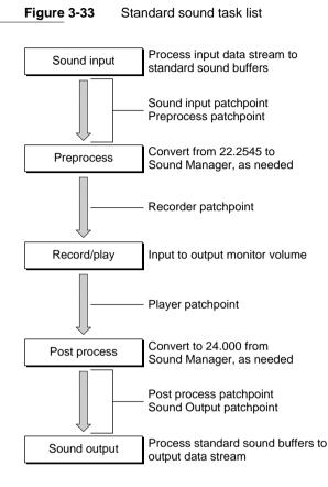
The sound input task takes the serial data stream from the DMA channel coming from the stereo A/D converter and converts it to DSP floating-point format. For 10 ms frames and 24 kHz sound, this takes the form of two 240-longword buffers. These buffers are established as ITBs by the DSP map structure associated with sound input.
