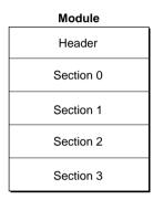
The header contains information about the entire module, such as its name, GPB information, and control flags. Also included in the header is a count of the number of sections in the module. This allows the module data structure to be of variable length.
