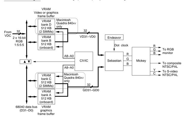
If the VRAM is configured as a single video frame buffer, it can all be used for graphics and the video input can be disabled. In this case, the CIVIC controls data access to VRAM from the following sources:
