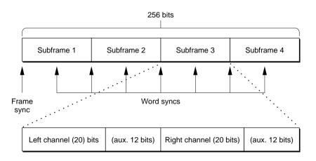
The signals singerSync, singerSerOut, and singerSerIn are clocked by the singerBitClk signal. The falling edge of the clock is used to clock the signals, and the rising edge is used to sample them. As shown in Figure 2-16, a frame sync is marked by a pulse two singerBitClk cycles wide; a word sync is marked by a pulse one singerSync cycle wide.
