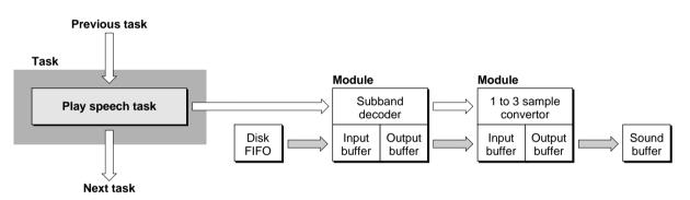
Notice that there are two types of connections in the diagram. First is the control flow, indicated with solid arrows. These are the connections that the DSP operating system follows to execute the real-time task list. The second type is the data flow connection, indicated by shaded arrows. In this example, data flows from the disk FIFO to the subband decoder module, from the decoder to the sample rate converter module, and from the converter module to the sound buffer.
