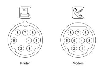
Either port can be independently programmed for asynchronous or synchronous communication formats up to 9600 baud, including AppleTalk. The printer port supports LocalTalk hardware protocols by means of a **LocalTalk Patch Chip (LTPC)**. In addition, the port marked "Modem" supports the full range of Apple GeoPort protocols, helping the computer communicate with a variety of ISDN and other telephone transmission means by using external pods.
