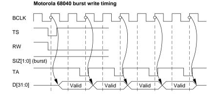
Cyclone alternate bus master burst write timing
