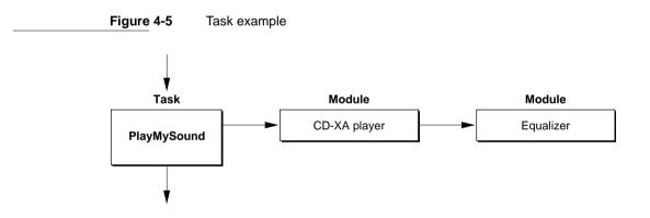
The task PlayMySound is shown installed in the task list. It points to two DSP modules. The first module, CD-XA player, is used to decompress CD-XA data from disk into PCM data. The equalizer module is used to adjust the tone quality of the sound, and feeds the results to the sound partial result buffer (PRB). The sequence of Real Time Manager calls that is necessary to set up and execute a task such as this is given in Table 4-3. Italicized calls are made only if necessary.
