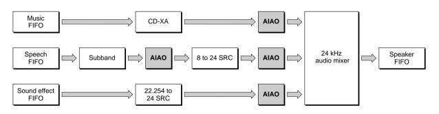
Figure 3-24 Code module data flow with AIAOs
