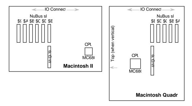
• Figure 2-1 Arrangement of the expansion slots
