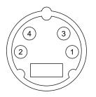
The ADB is a single-master, multiple-slave serial communications bus that uses an asynchronous protocol and connects keyboards, graphics tablets, mouse devices, and other devices to the computer. The custom ADB microcontroller drives the bus and reads status from the selected external device. For more information about the ADB, see *Guide to the Macintosh Family Hardware*, second edition.
