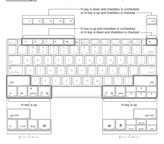
Figure 3-9 Embedded numeric keypad operation
