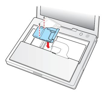
Once the RAM expansion module has been installed in the slot, the user must close up the computer by performing these steps in reverse order. Be careful to replace the shield plate properly so that the AirPort Card will fit.
