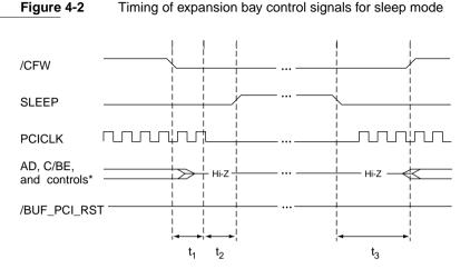
$t_1 = 16 \text{ ms min.}$  /CFW to clocks stopped  $t_2 = 16 \text{ ms min.}$  Clocks stopped to system sleep  $t_3 = 50 \text{ ms min.}$  Clocks started to clock valid
