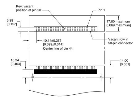
Note: Dimensions are in millimeters [inches].
