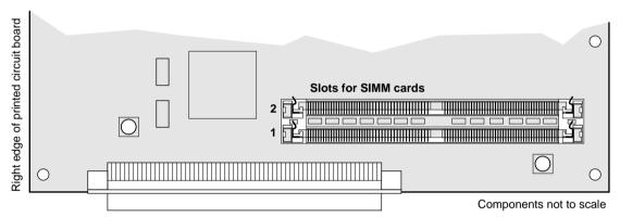
Back edge of printed circuit board
