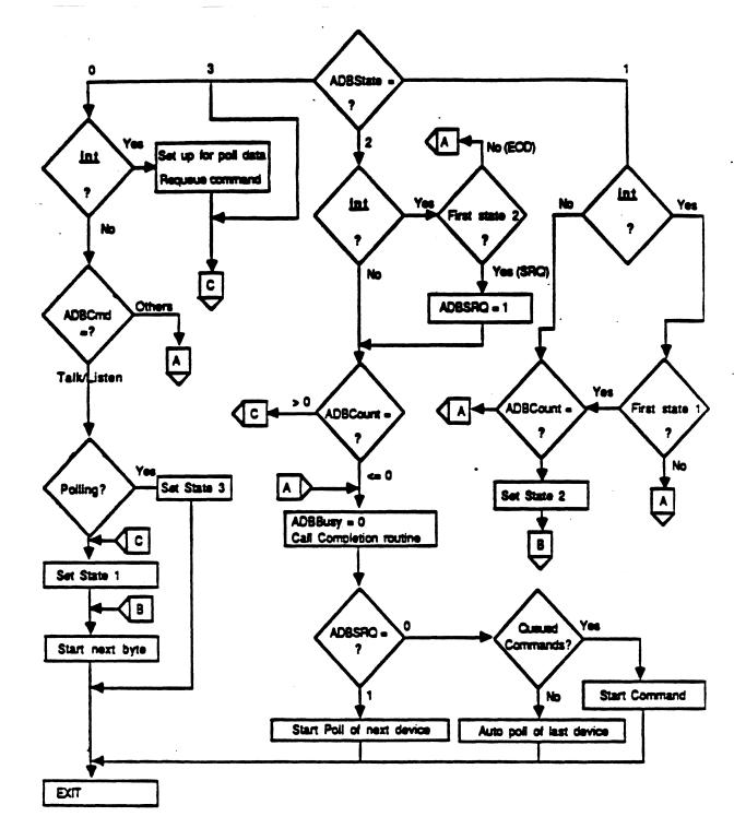
Figure 8. Shift-Register Interrupt Flowchart.
