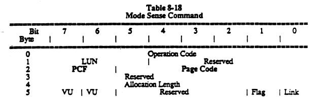
The MODE SENSE command (Table 8-18) provides a means for a target to report its medium, logical unit, target or peripheral device parameters to the initiator. It is a complementary command to the MODE SELECT command.
