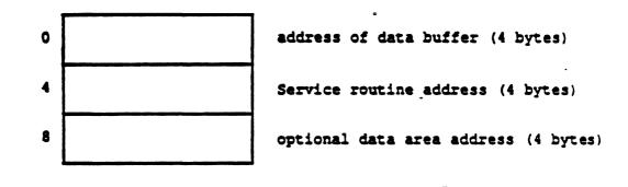
Figure 4. ADBOp Parameter Block
