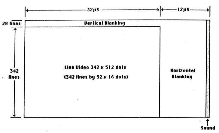
Live video: while the display is actively tracing a horizontal line of dots on the screen, video accesses to RAM (two words of data are read in each video access) alternate with three 68000 accesses.
