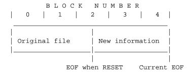
In this example, a SEEK to a record in the last half of block 2, block 3 or block 4 will cause problems.
